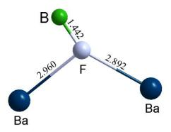
Bond length in conventional fluorooxoborates, B-F covalent interaction and Ba-F ionic interaction. Partial structure sketch map of alkaline-earth metal fluorooxoborate  $BaB_4O_6F_2$ . <sup>10</sup>
