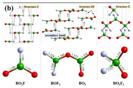
**Figure 2.** (a) Crystal structure of B<sub>2</sub>O<sub>2</sub>F<sub>2</sub> (I-X) with corresponding space group, structure units, and cell size. (b) Sketch map of I, III, X and their corresponding structure units; oxygen red, fluorine silvery, boron green.
