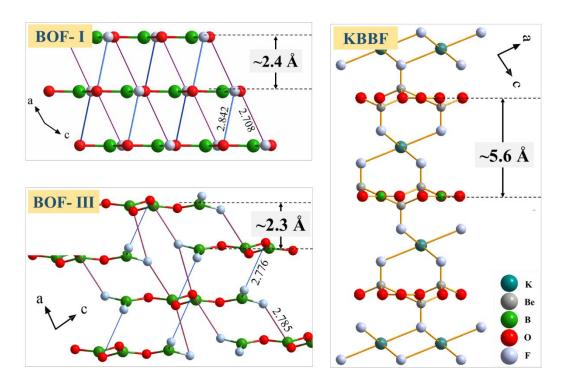
Predicted structure I, III with small interlayer space and B-F secondary bonds can effectively suppress the layering tendency.
