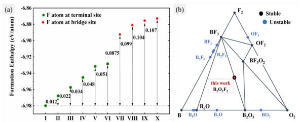
**Figure 1.** (a) Relative enthalpies of formation for different B<sub>2</sub>O<sub>2</sub>F<sub>2</sub> phases at ambient pressure. (b) Phase diagram of B-O-F system, phase diagram is generated with the help of Materials Project, <a href="https://materialsproject.org">https://materialsproject.org</a>.
