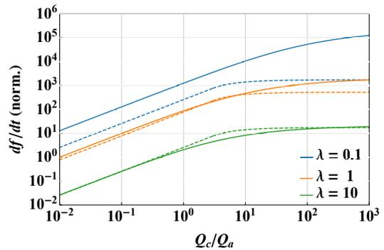
FIG. 6. Comparison of the scanning rate between the original (Eq. 4) and revised (Eq. 19) calculations as a function of normalized cavity quality factor,  $Q_c/Q_a$ , for three different values of  $\lambda$ , the relative noise contribution. The former and the latter estimations are represented by dashed and solid lines, respectively.
