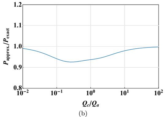
FIG. 7. (a) Comparison of the axion energy distributions between the exact description from Eq. A.1 and its Cauchy approximation in Eq. A.2 in terms of the axion kinetic energy  $u$ . The area below each distribution is normalized to unity and the peaks are matched. (b) Ratio between the two integrals in Eq. A.3 as a function of  $Q_c/Q_a$ .
