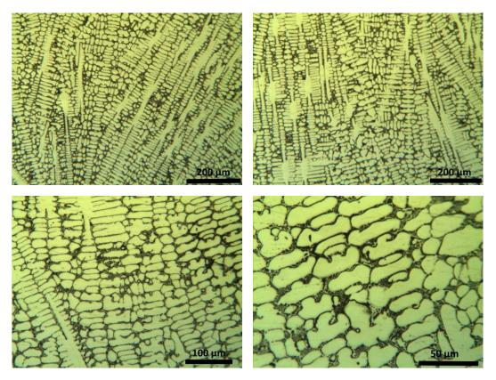
Figure 2. The as cast microstructure of alloy  $AI_{14}Co_{41}Cr_{16}Fe_{11}Ni_{18}$
