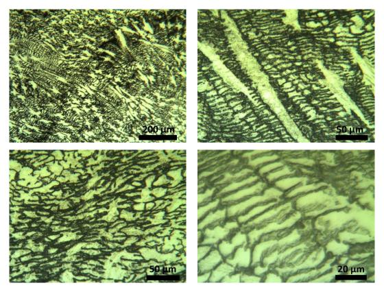
Figure 5. Observation of highly deformed areas on the investigated surface after compression test
