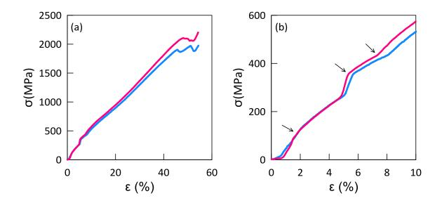
Figure 1. (a) The engineering compressive stress-strain curves for as-cast alloy  $AI_{14}Co_{41}Cr_{16}Fe_{11}Ni_{18}$  (b) observing three yielding points at small strains
