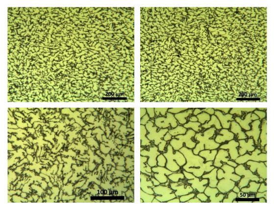
Figure 3. Distorted dendrites after compression test with no effect of twinning or SIM
