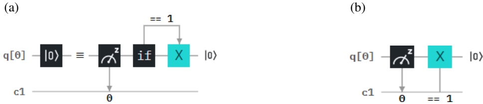
FIG. 3. Implementation of the qubit-reset gate for the IBM Q platform: (a) equivalence and schematic sketch, (b) typical implementation in the drag-and-drop circuit composer.
