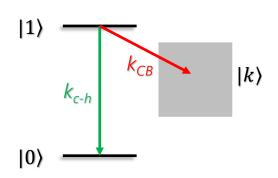
Supplementary Figure 3. Principle of CHC to determine lifetimes. The relative magnitude of the two rate constants  $k_{c-h}$  and  $k_{CB}$  determines the intensity of associated Auger features in the resonant photoemission map.
