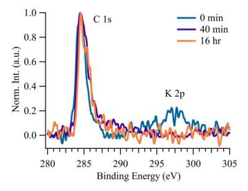
Supplementary Figure 1. XP spectra of C 1s and K 2p (normalized to C 1s) after K addition to bulk  $MoS_2$  (0 min) as a function of time, which demonstrates prompt K diffusion into the substrate.
