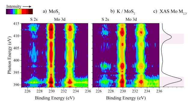
Figure 4. Resonant photoemission contour plots of a) as-cleaved and b) K-dosed MoS<sub>2</sub> monitoring the intensity changes of XP features Mo **3***d* and S **2***s* on resonance with Mo M<sub>2,3</sub>. c) XA spectrum of Mo M<sub>2,3</sub> with highlighted regions (pink) where resonantly enhanced photoemission may be expected in the RPES maps.
