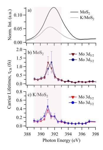
Figure 6. Carrier lifetimes of as-cleaved and K-dosed MoS<sub>2</sub>. a) Mo M<sub>3</sub> XA spectrum. Carrier lifetimes of b) MoS<sub>2</sub> and c) K/MoS<sub>2</sub> calculated from Mo **3***d* resonant intensities and their uncertainties, assuming  $\tau_{CB} = 1.24$  fs for MoS<sub>2</sub>.
