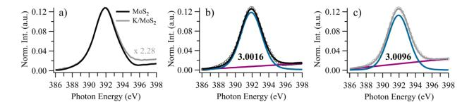
Supplementary Figure 2. XAS comparison of as-cleaved and K-dosed  $MoS_2$  with associated fits. a) Comparison of XA spectra on the Mo M<sub>3</sub> edge for  $MoS_2$  and K/MoS<sub>2</sub>. The latter is scaled and shifted for ease of comparison. XA spectral fits using a linear background and Voigt peak profile for b)  $MoS_2$  and c) K/MoS<sub>2</sub>. Nearly identical FWHM values (in eV) are identified in parts b) and c).
