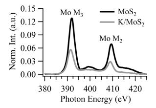
Figure 2. X-ray absorption spectra of cleaved (black) and K-dosed (gray) MoS<sub>2</sub> monitoring Mo M<sub>2,3</sub> absorption edges. Intensity is normalized with respect to the incident X-ray photon flux,  $I_0$ . Each XA spectrum shows the spin-orbit components of Mo M<sub>3</sub> ( $3p_{3/2}$ ) and M<sub>2</sub> ( $3p_{1/2}$ ).
