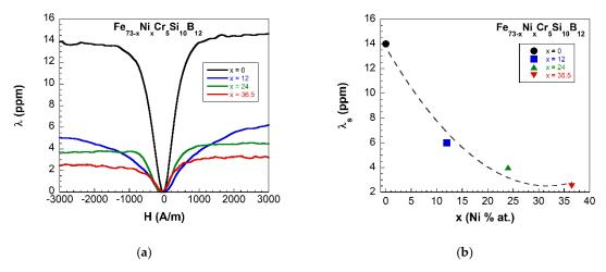
**Figure 4.** (a) Measured magnetostriction curves and (b) saturation magnetostriction values dependence with the composition of the samples showing ferromagnetism at room temperature (dashed line is a guide to the eye).
