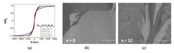
**Figure 8.** (a) Normalized hysteresis loops and Kerr microscopy images of samples: (b) x = 0 and (c) x = 12 at remanence. Black contrast indicates negative saturation along the field direction, while white contrast corresponds to positive saturation along the field direction.
