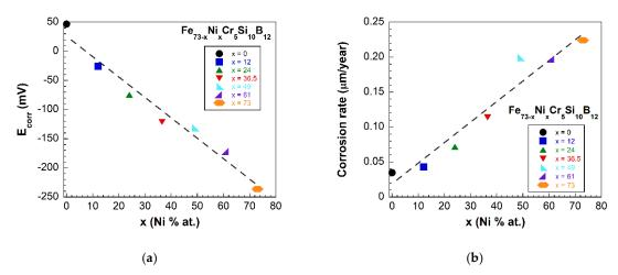
**Figure 7.** (a) Corrosion potential ( $E_{corr}$ ) and (b) corrosion rate values obtained from Tafel and  $R_P$  fittings of the LPR curves obtained for all the fabricated  $Fe_{73-x}Ni_xCr_5Si_{10}B_{12}$  samples (dashed lines are a guide to the eye).
