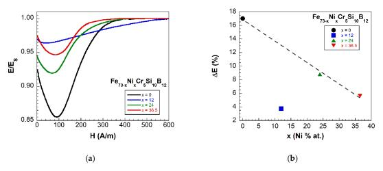
**Figure 5.** (a) Change of the Young modulus with the applied magnetic field (or  $\Delta E$  effect), and (b) measured  $\Delta E$  effect values dependence with the composition of the samples showing ferromagnetism at room temperature (dashed line is a guide to the eye).
