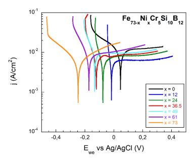
**Figure 6.** Potentiodynamic polarization curves of all the fabricated  $Fe_{73-x}Ni_xCr_5Si_{10}B_{12}$  samples, measured in a three-electrode cell in phosphate buffer solution (PBS) at 25 °C and pH 7.3.
