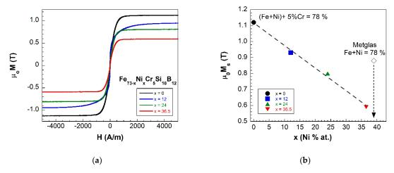
**Figure 2.** (a) Hysteresis loops of samples exhibiting ferromagnetic response at room temperature and (b) saturation magnetization value decrease as the Ni % at content increases in the composition (dashed line is a guide to the eye).
