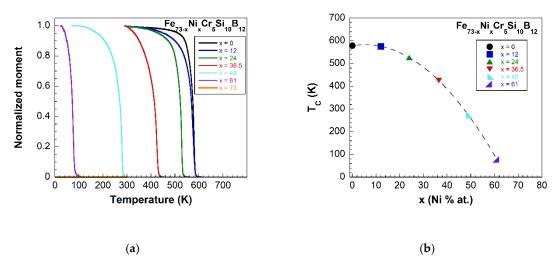
**Figure 3.** (a) Variation of the magnetization with the temperature for all the studied samples, and (b) Curie temperature dependence with the composition of the samples (dashed line is a guide to the eye).
