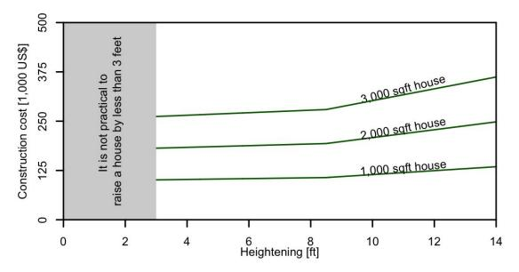
**Supplementary Figure 14:** Construction cost for three sample houses with sizes of 1,000, 2,000, and 3,000 ft<sup>2</sup>. The gray area indicates an elevation of fewer than three feet which we assume to be impractical. These cost estimates are adopted from the CLARA model. Units are in 2017 US\$ value
