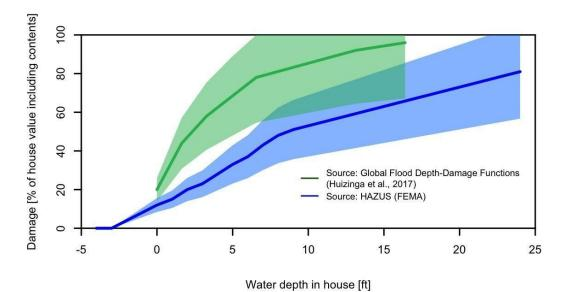
**Supplementary Figure 12:** Two depth-damage functions used in this study. The damage model in blue is obtained from FEMA HAZUS and the damage curve shown in green is obtained from combining multiple functions from HAZUS<sup>8</sup>. Shallow uncertainty in each function is represented by 30% uniform bounds (shown in light blue and green)
