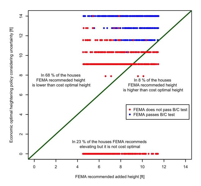
**Supplementary Figure 11:** The economic optimal elevation versus FEMA's recommendation. Each dot represents a house (a total of 1,000 houses). Red dots indicate that FEMA's recommended policy does not pass the cost-benefit test (i.e. the benefit is less than the cost). The diagonal green line is the 1:1 line
