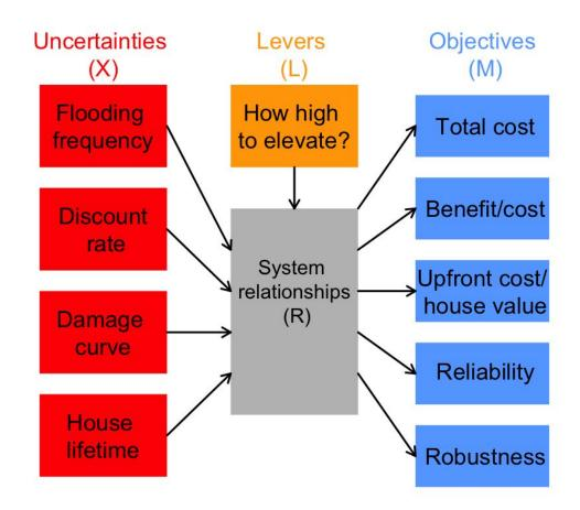
**Supplementary Figure 1:** An XLRM diagram that shows the decision framework. The orange element is the lever (L) (i.e. how high to elevate a house). Red components represent exogenous uncertain factors (X) that impact the decision and are out of control of the decision-maker. Objectives or metrics (M) represent how success is measured. System relationships (R) shows how levers and uncertainties translate into objectives
