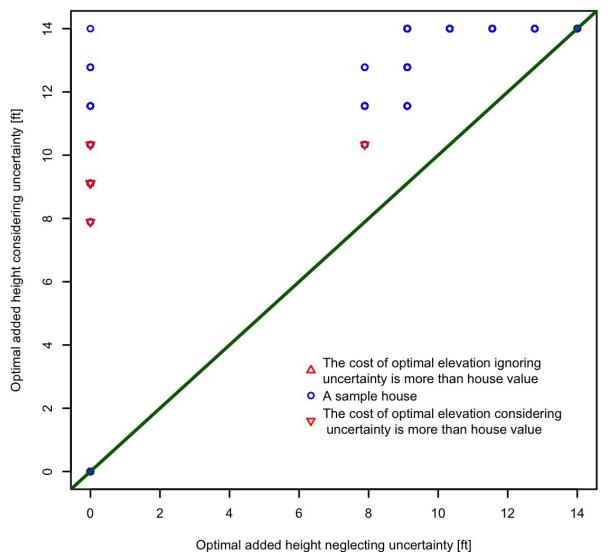
**Supplementary Figure 10:** Comparison of economically-optimal elevations under two assumptions of ignoring-uncertainty and considering-uncertainty. Each point represents a house. Houses in which one or both of the optimal elevations are more than house value are indicated by red
