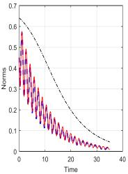
Fig. 6. Estimation of solution norms for Duffing-like and Van der-Pol-like models. Blue, red and black lines plot timehistories of the corresponding norms of solutions and their estimate, respectively.
