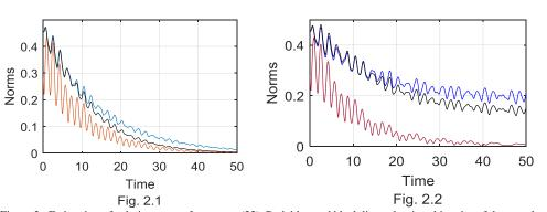
our simulations throughout. The estimations of the norms of solutions to (33) are shown in Fig.2.1 and Fig.2.2, where red, blue, and black lines plot time-histories of the actual norms of solutions and
