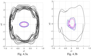
Fig. 4. Estimation of stability/trapping regions. Figures 4.1a-4.3a plot approximate boundaries of stability/trapping regions of (33) in projections on  $x_1 - x_2$  - plane. Black lines are developed in simulations of (33) in reverse time. Blue-lines are developed in simulations of (20) and magenta-lines are developed through utility of either (26) (Fig. 4.1a) or (31) (Figs. 4.2a and 4.3a).
