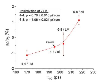
Figure 6. Relative change of electrical resistivity during AA for 10 s measured for two alloys and two media (LM, oil). Black points are individual measurements, red points are averages. The data is related to positron lifetimes derived from Figure 2a and Figure 3.
