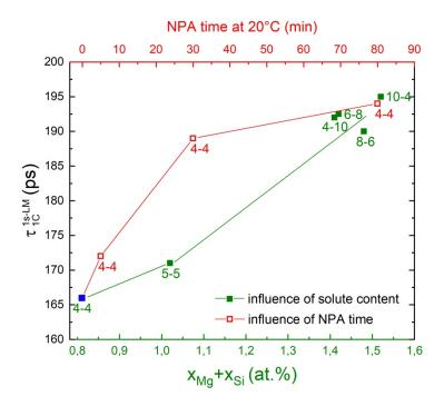
Figure 4.  $\tau_{1C}$  after 1 s of AA in LM for various alloys with different Mg and Si contents (full symbols). Data for alloys 4-4 and 6-8 is the same as in Figure 2a (lowest value chosen) and Figure 3. For alloy 4-4, an additional NPA step (5, 30 or 80 min) has been included before AA (open symbols).
