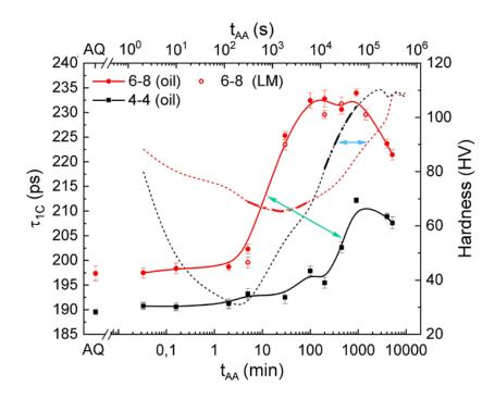
Figure 5. Hardening of alloy 4-4 and 6-8 at 180 °C in oil (and in LM for some cases). The thin broken lines represent the positron lifetimes  $\tau_{1C}$  taken from Figure 2a and Figure 3. On these lines, the dash-dotted sections emphasise the regions of main hardening. The double-sided arrows show the offset between main hardening and final increase of  $\tau_{1C}$  for the two alloys.
