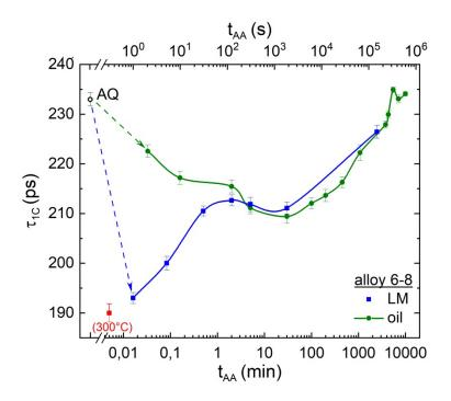
Figure 3. Evolution of the one-component positron lifetime  $\tau_{1C}$  in alloy 6-8 as a function of AA time at 180 °C in different heating media. The red symbol corresponds to 0.3 s annealing at 300 °C.
