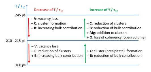
Figure 7. Alternative mechanisms governing the change of the averaged ( $\bar{\tau}$ ) or one-component positron lifetime ( $\tau_{1C}$ ) during ageing. '+' and '-' denote an increase or decrease of a specific contribution. In this paper, vacancy (V) loss, clustering (C), loss of coherency (O) and the change of bulk annihilation (B) is discussed. Change of Mg content (Mg) governs natural ageing [8] and is not relevant here.
