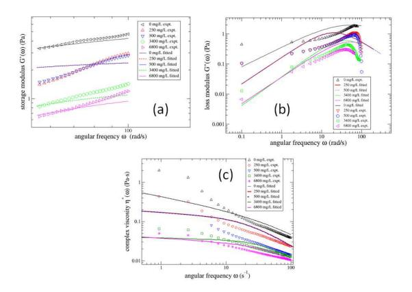
Figure 3: Salinity variation:(a)Comparison between experimental and calculated storage modulus using Maxwell Model.<sup>30</sup> (b)Comparison between experimental and calculated loss modulus using Maxwell Model.<sup>30</sup> (c)Comparison between experimental and calculated complex viscosity using Maxwell Model.<sup>30</sup>
