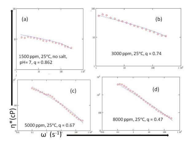
Figure 7: Variation of complex viscosity versus angular frequency for different polymer concentrations at constant temperature of  $25^{\circ}$ C, pH=7 and zero salinity, (a)1500 ppm (b)3000 ppm (c) 5000 ppm (d) 8000 ppm. Comparison between experiment and theory is good in each case.<sup>32</sup> The order of the fractional derivative decreases with increase in concentration as displayed in the graph.
