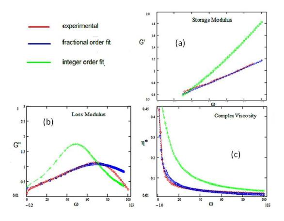
Figure 2: The rheological properties of HPAM obtained from experimental data compared with calculated values using Maxwell's Model using integer derivative and fractional derivative calculus.<sup>30</sup> (a) Storage modulus (b)Loss modulus (c)Complex viscosity. In all cases, the fractional derivative calculus fitted best the experimental data.
