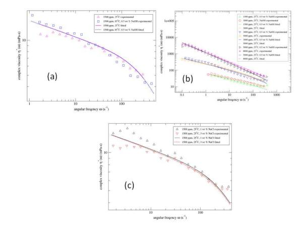
Figure 9: Variation of complex viscosity versus angular frequency for different combinations of *complementary conjugates*. Experimental data from Choi e.t al. have been modelled.<sup>32</sup> (a)Higher temperature is offset by a suitable increase in pH. (b)Effect of increased polymer concentration offset by lower the pH value. (c)Variations in salt concentration alone cannot offset small changes in concentration.
