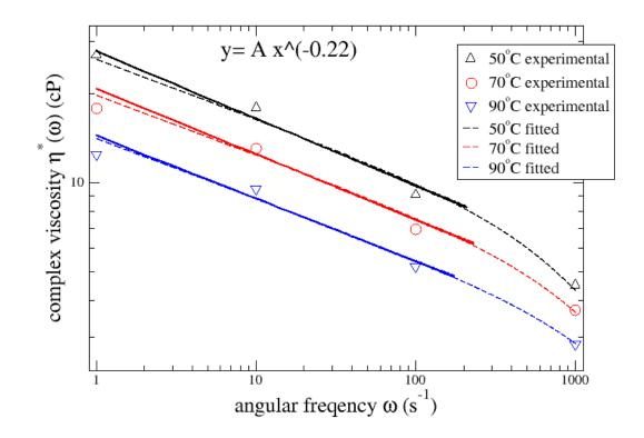
Figure 6: Variation of complex viscosity versus angular frequency for different temperatures: comparison between experiment and theory.<sup>31</sup> For angular frequencies  $\sim 120 \ s^{-1}$ , the variation follows a power law with exponent of 0.22 for every temperature. The power law fit is shown by thick solid line.
