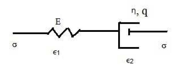
Figure 1: Schematic Maxwell model. E is the spring constant and  $\eta$  represents the viscosity of the fluid in the dashpot. For a stress  $\sigma$ ,  $\epsilon_1$  is the strain the the spring and  $\epsilon_2$ , that in the dashpot.
