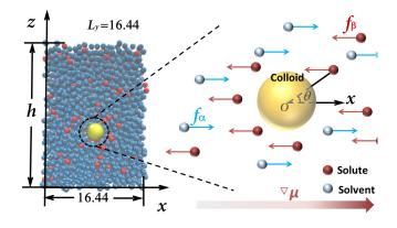
**Fig. 1** The left figure shows a colloidal particle embedded in a mixture of solvent (blue) and solute (red) particles. The right-hand figure shows the gradient in the chemical potential of solvent and solute particles, represented by "color" forces acting on these particles. The strength of these forces is such that the average force on a fluid element in the bulk of the liquid vanishes, because the bulk pressure is constant throughout the system.
