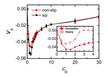
**Fig. 3** Fluid velocity  $v_x$  versus solute-colloid (isotropic) interaction strength  $\varepsilon_B$  for slip (red; circles) and non-slip (black; squares) boundaries. The inset shows a comparison of the non-slip data in the regime  $\varepsilon_B < 4.0$  (solid) to the Derjaguin–Anderson theory (Eq.7, dashed).
