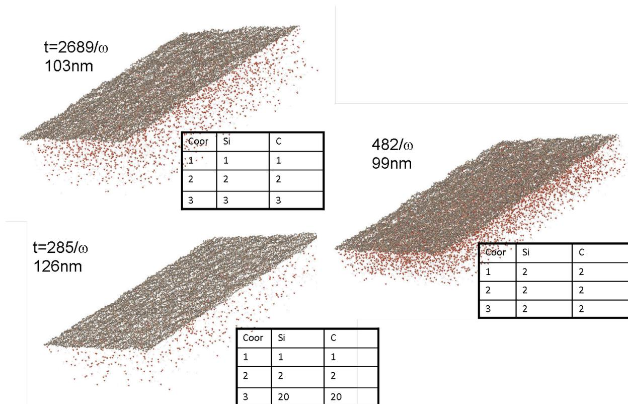
**Fig. 7** Simulation snapshots obtained starting from a flat 3C-SiC substrate for three different choices of the deposition parameters (in  $\omega$  units) and  $P_{\text{transZigZag}}=1$ . The quote relative to the initial substrate height obtained in the simulated evolution is indicated. Vacancy type defects are visible in all the graphs. They are in the bulk crystal whist the vapor phase is in the other side with respect to the surface.
