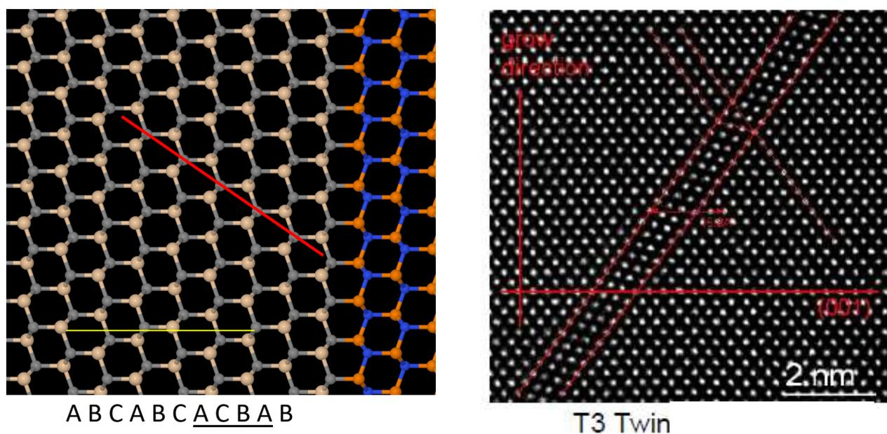
**Fig. 2** Atomic representation (Left-hand panel) and HRTEM (right-hand panel) image of a "Micro Twin like" SF in 3C-SiC. The faulted stacking sequence of the Si-C dimers along a  $\langle 111 \rangle$  direction with respect to the ideal ABC ABC ABC...one is indicated. The red line is a guide for the eye, highlighting the maintained epitaxial order in the two semi-spaces separated by the defect.
