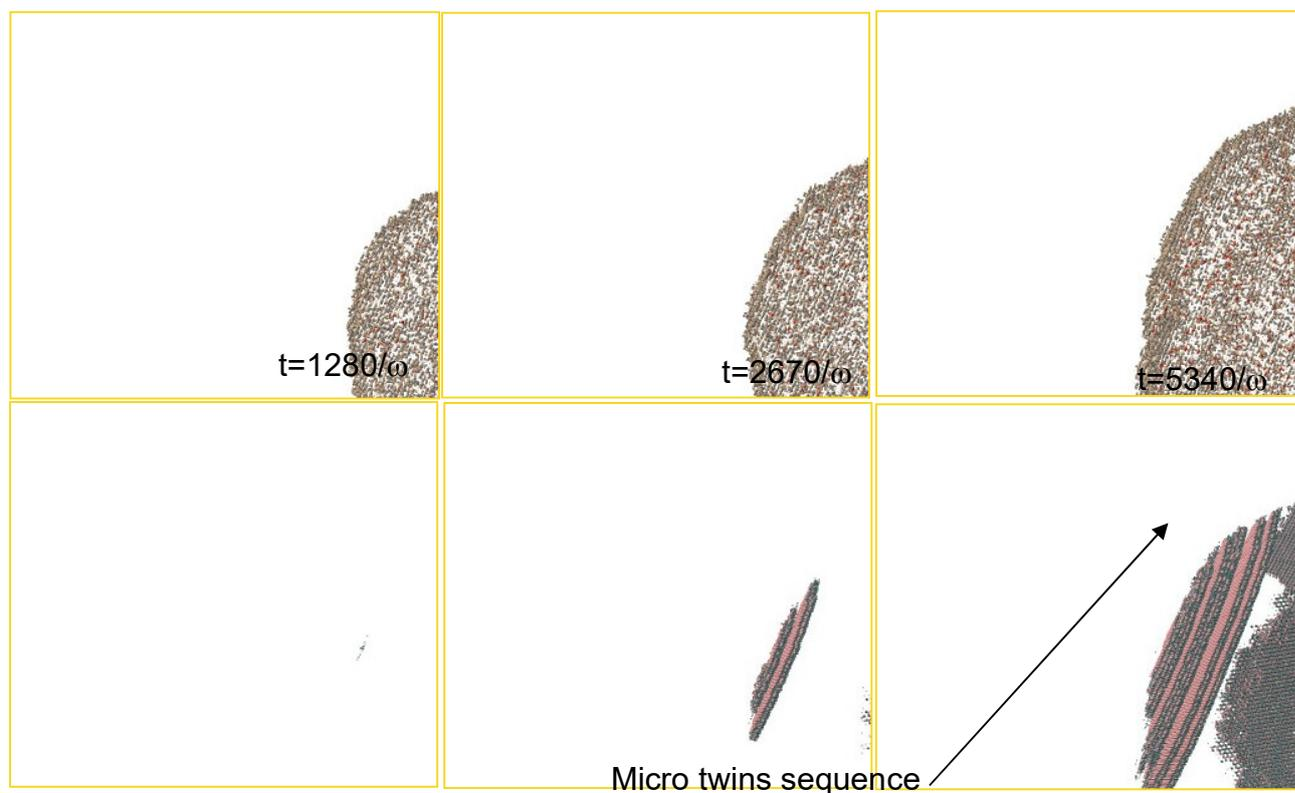
**Fig. 10** Simulation snapshots of the growth of a 3C-SiC nano-crystal starting from a cubic seed with facets oriented in the  $\langle 100 \rangle$  direction. In the bottom panel, atoms which are not epitaxially ordered are shown. The deposition parameters (in  $\omega$  units) are equal to the case reported in fig. 7 top panel ( $P_{\text{transZigZag}}=0.5$ ).
