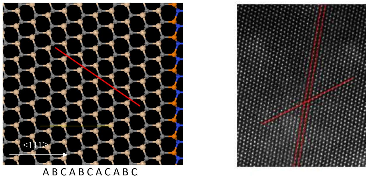
**Fig. 1** Atomic representation (Left-hand panel) and HRTEM (right-hand panel) section of an "intrinsic" SF in 3C-SiC. The faulted stacking sequence of the Si-C dimers along a  $\langle 111 \rangle$  direction with respect to the ideal ABC ABC ABC...one is indicated. The red line is a guide for the eye, highlighting the breaking of the epitaxial order in the two semi-spaces separated by the defect: The atoms are displaced by  $1/3$  of the Si-C bond distance.
