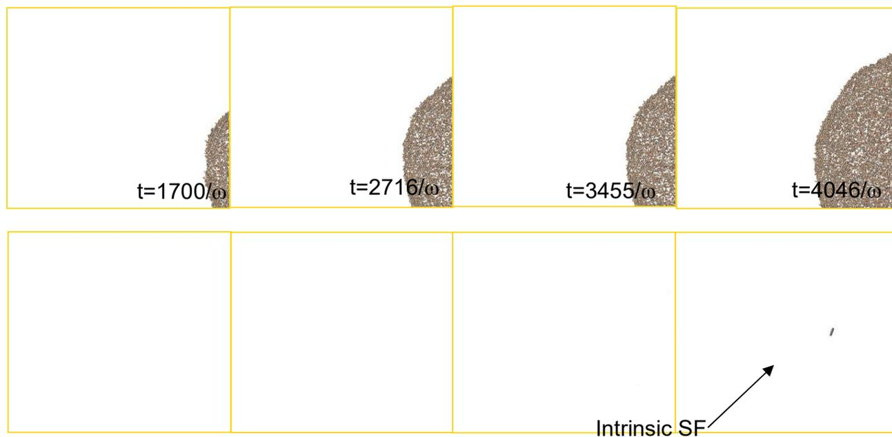
**Fig. 9** Simulation snapshots of the growth of a 3C-SiC nano-crystal starting from a cubic seed with facets oriented in the  $\langle 100 \rangle$  direction. In the bottom panel, atoms which are not epitaxially ordered are shown. The deposition parameters (in  $\omega$  units) are equal to the case reported in Fig. 5 top panel ( $P_{\text{transZigZag}}=0.8$ ).
