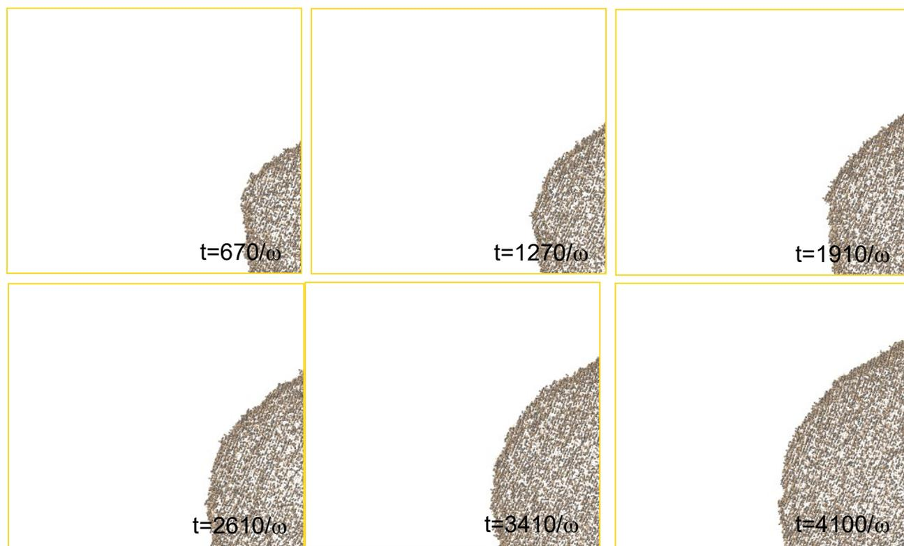
**Fig. 8** Simulation snapshots of the growth of a 3C-SiC nano-crystal starting from a cubic seed with facets oriented in the  $\langle 100 \rangle$  direction. The deposition parameters are equal to the case reported in Fig. 5 top panel.
