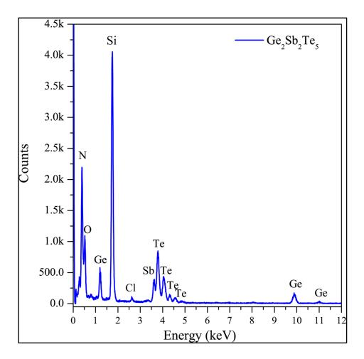
**FIG. 3**. X-ray energy dispersive spectrum of as-deposited 30 nm GeSbTe film showing significant oxygen content.
