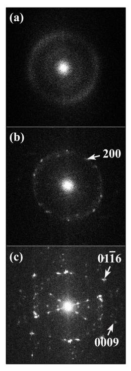
**FIG. 2.** Power spectrum from STEM-HAADF images of (a) as-deposited GST film at room temperature, heated at (b) 130  $^{\circ}$ C and (c) 200  $^{\circ}$ C. The phase transformation from amorphous to metastable face-centered cubic (fcc) phase is observed at 130  $^{\circ}$ C and the second transformation from fcc to a stable hexagonal closed pack (hcp) phase at 200  $^{\circ}$ C during in-situ heating in the microscope under vacuum.
