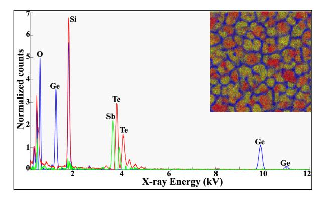
**FIG. 6.** XEDS profile and composite image (inset) of  $Ge_2Sb_2Te_5$  including oxygen after heat treatment at 200 °C. The inter islands regions are enriched in Ge and O. The field of view for the composite image is 125 nm.
