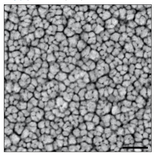
**FIG. 1**. Low-magnification scanning transmission electron microscope high-angle annular dark field (STEM-HAADF) image of  $Ge_2Sb_2Te_5$  thin film of 30 nm thickness deposited by sputtering. The morphology shows island like nature of the sputtered film in as-deposited condition. The scale bar is 50 nm.
