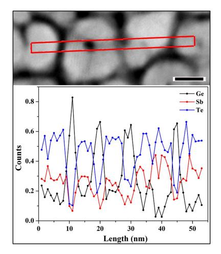
**FIG. 5**. STEM-HAADF image and XEDS line profiles (red line from left to right) of Ge, Sb and Te after heat treatment at 200 °C. The scale bar for the image is 10 nm.
