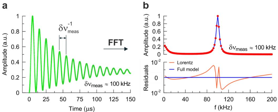
**Figure 2 Transient cavity response to single-mode, non-resonant excitation.** (a) Simulated buildup signal for  $\delta\nu_{meas} = 100$  kHz and a driving field switch-on time of 50 ns. For clarity, the initial 150  $\mu$ s of the signal is shown.
