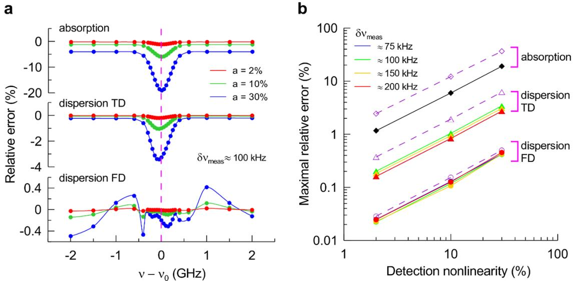
**Figure I Influence of detection system nonlinearity on the spectrum accuracy.** (a) Relative systematic differences between absorptive/dispersive spectra obtained from ring-down/buildup signals simulated with and without nonlinearity of the amplitude for corresponding nonlinear factors  $a$ : 2%, 10% and 30%. The buildup signals were analyzed in the time and frequency (as a power spectrum) domains leading to spectra denoted as
