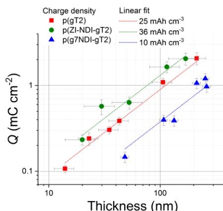
Figure S39. Charge density as a function of film thickness for the p-type and n-type polymers.
