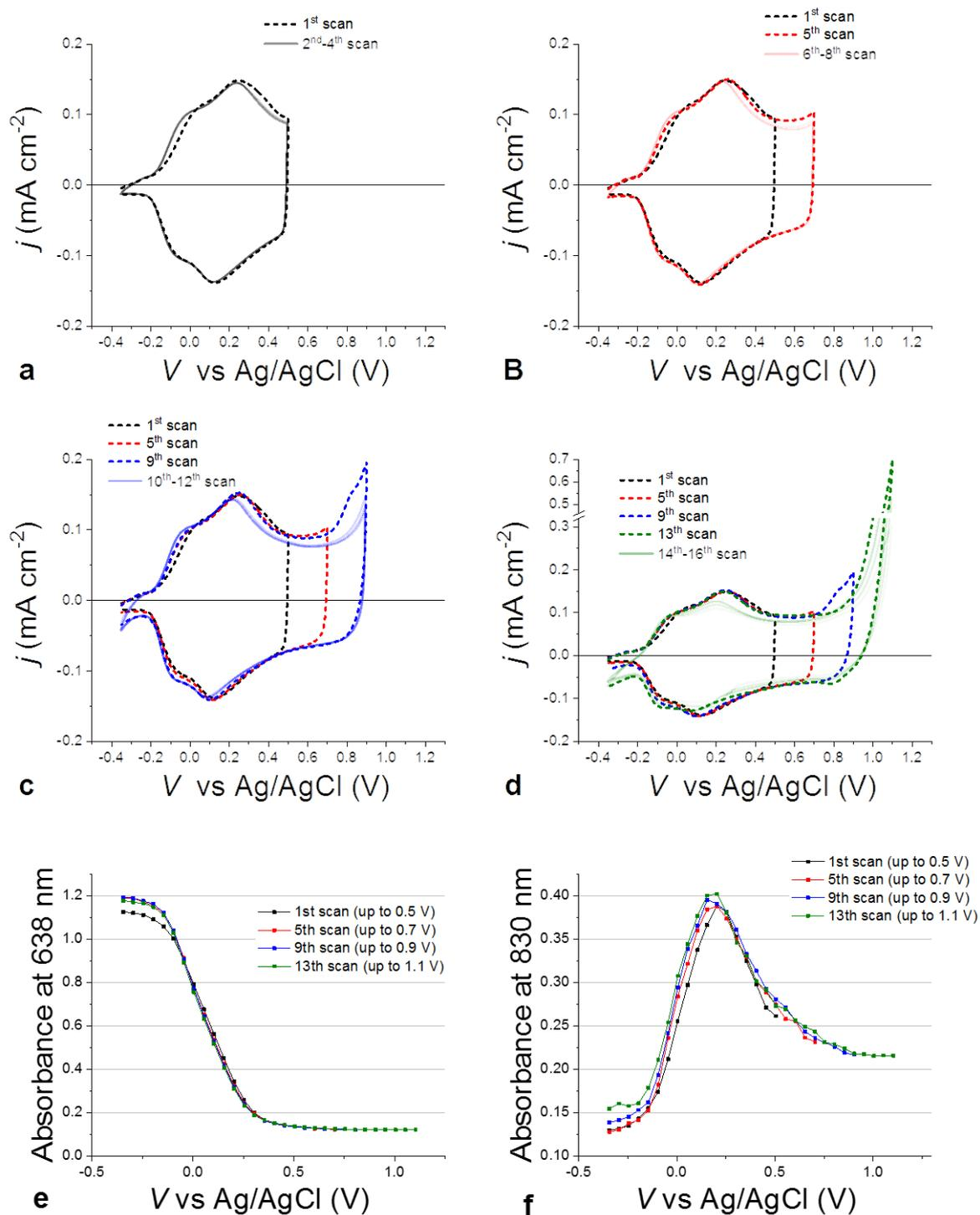
Figure S34. Electrochemical charging and reversibility of p(gT2) on FTO glass. (a) to (d) consecutive cyclic voltammometry measurements performed on a p(gT2) polymer film deposited on FTO in 0.1 M
