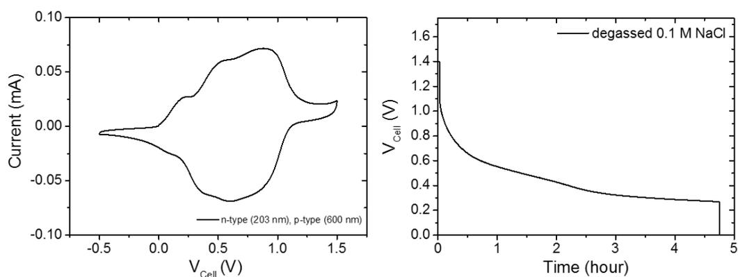
Figure S47. (a) CV of the electrochemical cell before the retention experiment. (b) Retention experiment where a voltage of 1.4 V is applied for 100 s to charge the cell followed by monitoring the potential for 286 min at open circuit. A degassed 0.1 M NaCl solution is used as the supporting electrolyte.
