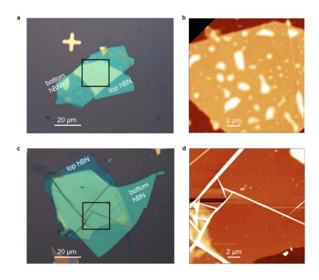
Figure S2: Optical images and AFM of hBN-encapsulated samples. (a) Optical image (100x magnification) of a hBN/QC-TBG/hBN with considerable interface contamination. (b) Atomic force microscopy (AFM) over the square area indicated in (a), highlighting numerous blisters. (c) Optical image (100x magnification) of a hBN/QC-TBG/hBN with successful interface cleaning. (d) AFM over the square area in (c), showing large and flat bubble-free areas.
