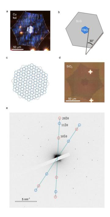
**Figure 1.** (a) Dark field optical microscopy image of a typical QC-TBG grown by CVD on Cu foil. (b) Schematic structure of the sample shown in (a), with the two superimposed concentric hexagons rotated by 30°. (c) Sketch of the crystal structure of the 12-fold rotationally symmetric QC-TBG. (d) Bright field microscopy image of a QC-TBG after transfer by semi-dry method on
