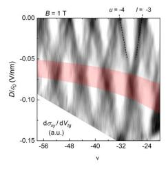
Figure S7: LLs crossings in D1 and interlayer capacitance. Zoom in main text Figure 3c, highlighting LLs crossings measured in D1 at B = 1 T. The displacement field D results in a density mismatch  $\Delta n$  and an electrostatic potential difference  $\Delta V$  between the layers, according to D = 1
