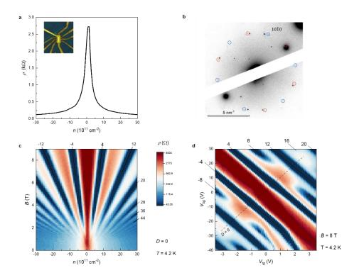
Figure S8: Magnetotransport on device D3, TBG from exfoliated graphene flakes. (a) Resistivity of device D3 as a function of carrier density at D = 0. The carrier mobility is ~40 x  $10^3$  cm<sup>2</sup>/Vs. Inset; optical microscopy image of D3, made from hBN-encapsulated TBG obtained by artificial stacking of two exfoliated single-layer graphene. (b) Representative SAED image for
