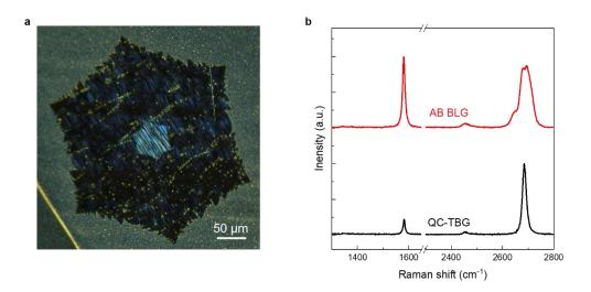
**Figure S1: Optical image and Raman of CVD AB bilayer graphene.** (a) Dark field optical microscopy image of an AB-stacked bilayer graphene crystal on Cu foil. (b) Representative Raman spectrum of AB bilayer graphene (red line), after transferring to SiO<sub>2</sub>/Si; a spectrum of QC-TBG (black) is shown for comparison.
