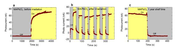
Figure 8 – Electro-optical response of irradiated MAPbCl<sub>3</sub> device. The photo-response before and right after absorbed 57 Sv  $H^*(10)$  ambient total  $\gamma$ -dose is unchanged, showing radiation hardened behaviour of the MAPbCl<sub>3</sub> device.(a and b). c) The photo-response of the device shows no degradation even after one-year shelf time.
