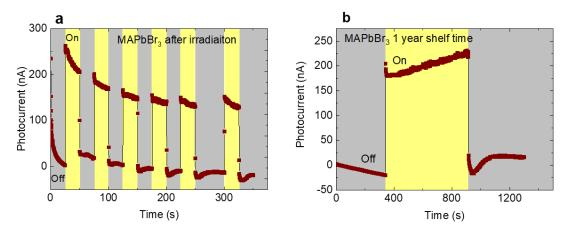
Figure 7 – Electro-optical response of irradiated MAPbBr3 device. There is a clear photo-response right after absorbed 57 Sv  $H^*(10)$  ambient total  $\gamma$ -dose (a). b) The photo-response of the device shows no degradation even after one-year shelf time.
