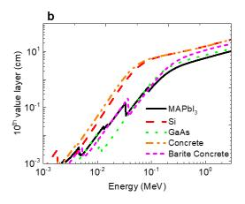
Figure 3: Radiation shielding properties of MAPbI<sub>3</sub> a) Comparison of normalized dose rate shielded by 10 cm thick slab of MAPbI<sub>3</sub>, BA type barite concrete and ordinary concrete calculated by MCNP. Different colours represent initial photon energy. b) Calculated 10<sup>th</sup> value layer, i.e. the layer where over 90% of the radiated energy is absorbed, for MAPbI<sub>3</sub>, Si and GaAs (materials for photon-detection) and various concretes used as shielding materials.
