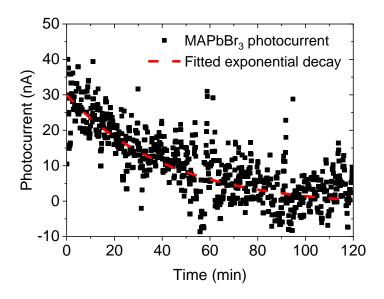
Figure 9 – Gammavoltaic effect of MAPbBr<sub>3</sub> exposed to the  $\gamma$  radiation of a shutdown nuclear reactor. The  $\gamma$ -induced photocurrent follows the decreasing  $\gamma$ -dose rate with  $\tau^{PC}$ =2555±140 s time constant (extracted from the fit in red dashed line).
