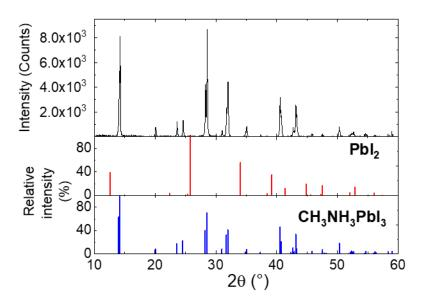
Figure 5 – Powder X-ray diffractogram of MAPbI3 after irradiation
