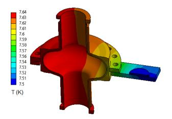
FIG. 5. Temperature distribution on the cavity surface and Cu plate with 5 W rf heat load and 0.58 W static heat load, calculated with ANSYS.
