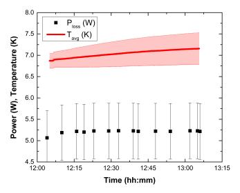
FIG. 4. Average temperature of the cavity outer surface while operating the conduction cooled cavity in cw mode with a constant dissipated power of 5 W for 1 h with no indication of thermal instability. The width of the shaded area corresponds to the standard deviation.
