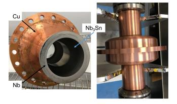
FIG. 1. Pictures of the multi-metallic SRF cavity. The length of the cavity from flange to flange is 31.8 cm and the electroplated Cu ring at the equator is 25.4 cm in diameter and 1.27 cm thick.
