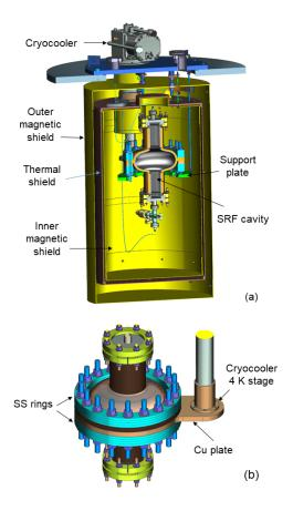
FIG. 2. Cross-section of the 3D model of the cavity-cryocooler the test stand (a) and detail of the cavity connection to the cryocooler 4 K stage (b). The test stand has a 61 cm diameter top plate and it is 93 cm in height.
