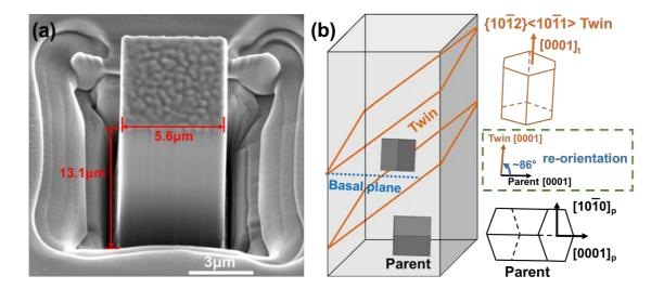
Fig. 1. (a) Representative micropillar of 5 x 5  $\mu$ m<sup>2</sup> cross-section. (b) Schematic of the orientation relationship between the parent and twin regions in the micropillar. The parent crystal is reoriented by ~86° by twinning.
