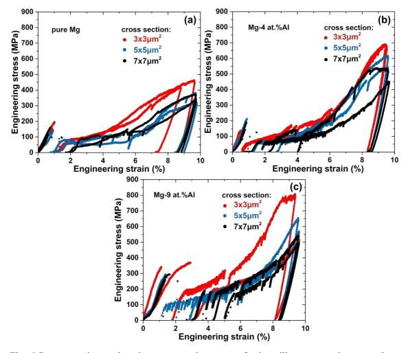
Fig. 6 Representative engineering stress-strain curves of micropillar compression tests along  $[01\overline{10}]$  direction in micropillars with lateral cross section in the range 3x3  $\mu$ m<sup>2</sup> to 7x7  $\mu$ m<sup>2</sup>. (a) Pure Mg, (b) Mg-4 at.%Al alloy and (c) Mg-9 at.%Al alloy.
