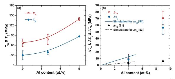
Fig. 9 (a) CRSS for twin nucleation,  $\tau_n$ , and growth,  $\tau_g$ , measured in micropillars of 7x7  $\mu m^2$  cross-section as a function of Al content. (b) Increase of the CRSS for twin nucleation,  $\tau_n$ , and growth,  $\tau_g$ , as a function of the Al content. Experimental data of the increase of CRSS for basal slip [21] and the first-principle predictions of the effect of Al content on the CRSS for twin growth [51] and basal slip [53] are also plotted for comparison.
