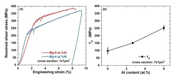
Fig. 10 (a) Representative resolved shear stress – e strain curves of micropillars of 5x5 and 7x7  $\mu$ m<sup>2</sup> cross-section of Mg-4 at.%Al, and Mg-9 at.%Al. (b) CRSS to activate pyramidal dislocation slip in Mg, Mg-4 at.%Al and Mg-9 at.%Al. The results for pure Mg are obtained from [30,32].
