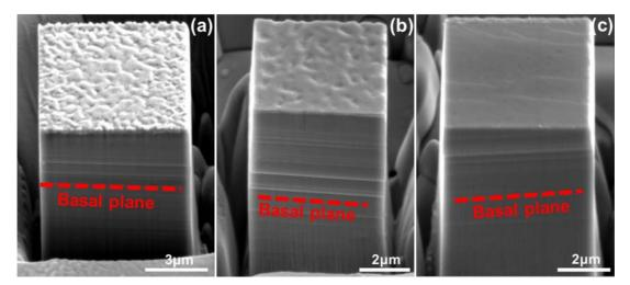
Fig. 7 SEM micrographs of the  $5x5 \ \mu\text{m}^2$  micropillars deformed up to 10%. (a) pure Mg, (b) Mg-4 at.%Al alloy and (c) Mg-9 at.%Al alloy. Slip traces along the basal plane of the twinned region are indicated by the red dash lines.
