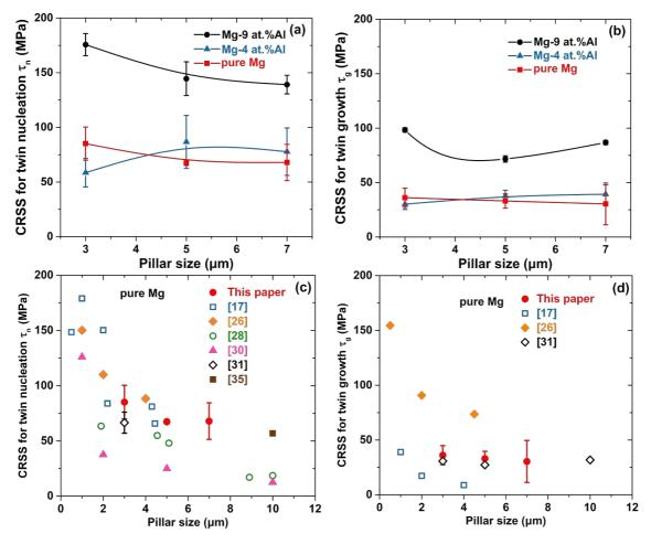
Fig. 8 (a) CRSS for twin nucleation ( $\tau_n$ ) as a function of the micropillar lateral dimension and Al content. (b) CRSS for twin growth ( $\tau_g$ ) as a function of the micropillar lateral dimension and Al content. (c-d) Effect of micropillar dimension on the CRSS for twin nucleation and growth for pure Mg. Results from this investigation and from the literature [17,26,28,30,31,35].
