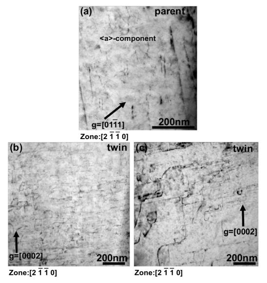
Fig. 5. (a) Applied strain 1%. <a> dislocations in the prismatic plane within the parent region,  $g=[01\overline{1}1]_p$ . (b) Applied strain 1%. <c> dislocations in the twinned region,  $g=[0002]_t$ . (c) Applied
