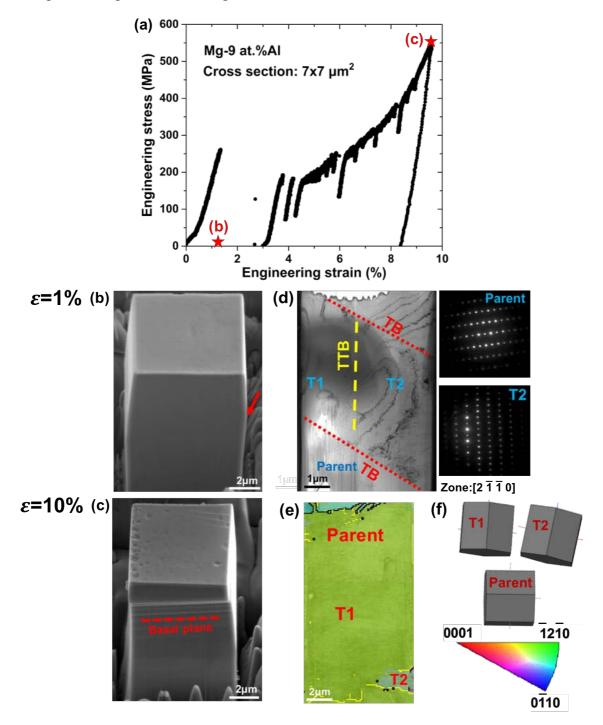
Fig. 4 (a) Representative engineering stress-strain curve of a Mg-9 at.%Al micropillar of  $7x7 \mu m^2$  deformed in compression along the [0110] orientation. (b) SEM micrograph of the deformed micropillar after the load drop at ~ 1% strain. (c) *Idem* at 10% strain. (d) TEM micrograph of the thin lamella extracted from the micropillar in (b), including the diffraction patterns of the parent
