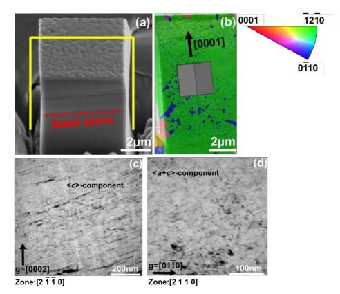
Fig. 11 (a) SEM micrograph of the Mg-4 at.%Al micropillar deformed along the [0001] direction. (b) *t*-EBSD maps of a thin lamella extracted from the micropillar in (a). (c) TEM micrographs of that lamella under the condition g=[0002] to reveal the  $\langle c \rangle$  dislocations. (d) Same as (c) observed under  $g=[01\overline{10}]$  to reveal  $\langle a \rangle$  dislocations.
