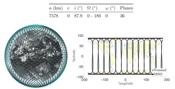
Figure 7: The initial conditions of the nominal and MiSO variants of the OneWeb LEO constellation (left), as well as their corresponding ground tracks (right).
