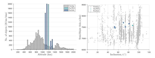
Figure 6: Altitude distribution (*left*) and (i, a) scatter plot (*right*) of the OneWeb LEO and SpaceX Starlink mega-constellations, as obtained from FCC filings no. SAT-LOI-20160428-00041 and SAT-MOD-20181108-00083, respectively, against the background cataloged satellites and debris in low-Earth orbit. ('Norad Resident Space Object Catalog. www.space-track.org. Assessed 27 Nov. 2019)
