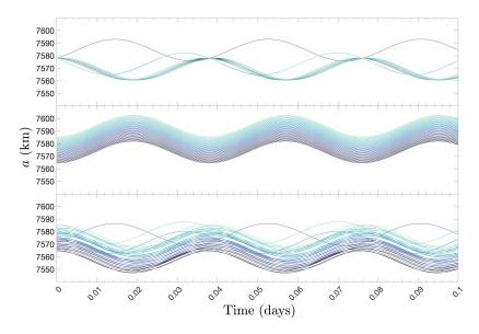
Figure 11: Comparison of the evolution of the osculating semi-major axis of a satellite in each plane of the nominal (top), MiSO (middle), and control case (bottom) configurations of the OneWeb LEO constellation.
