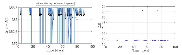
Figure 15: Close approaches within the Starlink MiSO satellites only occur when the difference in  $\omega + M$  of the target and field satellites is near zero. As the orbits become more perturbed from their initial configuration, the frequency with which this occurs becomes increasingly less consistent.
