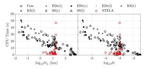
Figure 2: CPU time for 18-year integrations of a LEO against error in orbital elements. Black and red circles denote Cowell's method and STELA propagations, respectively, and other symbols represent various regularized formulations. Adapted from Amato et al. (2019), to which we refer for further details.
