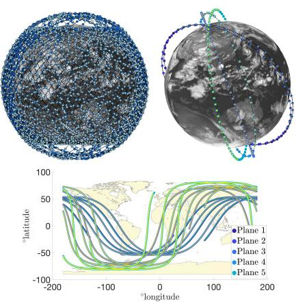
Figure 8: The initial conditions of the nominal and MiSO variants of the SpaceX Starlink constellation (*top*), as well as their corresponding ground tracks (*bottom*). Note that only the ground tracks of one plane in each shell, as depicted in the *top-right* panel, is shown.
