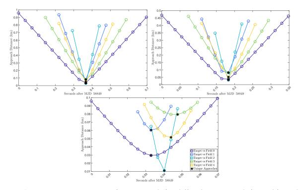
Figure 4: Integration output time steps of 0.0367 seconds (*top left*) and 0.0183 seconds (*top right*) are able to resolve a close approach of 0.0310 km, while an output time step of 0.0037 seconds (*bottom*) can resolve a close approach of 0.0109 km.
