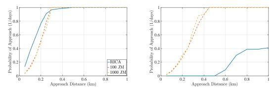
Figure 12: Comparison of the collision probability of the OneWeb nominal (*left*) and MiSO (*right* configurations.
