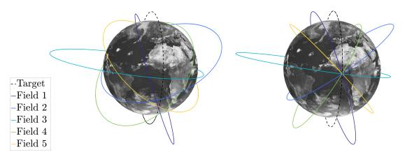
Figure 3: The initial orbits (*left*) at the epoch MJD 58834 and final orbits (*right*) at MJD 58849, the time of manufactured collision, for the **RICA** example objects of Table 1.
