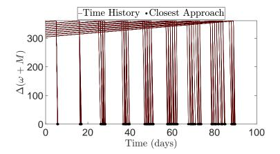
Figure 10: Close approaches within the OneWeb MiSO satellites only occur when the difference in  $\omega + M$  of the target and field satellites is zero. As the orbits become more perturbed from their initial configuration, the frequency with which this occurs becomes increasingly less consistent.
