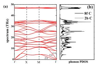
FIG. 2: (a) Phonon band structures along high symmetry path:  $\Gamma(0,0,0)$ -X(0.5,0,0)-M(0.5,0.5,0)- $\Gamma(0,0,0)$ , and (b) phonon density of states of clathrate graphene.
