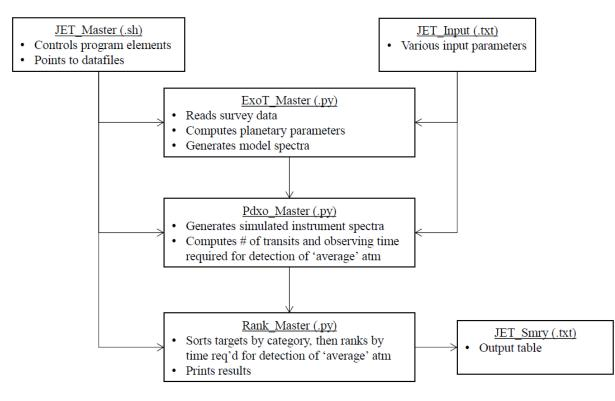
Figure 1. Top level JET program architecture.
