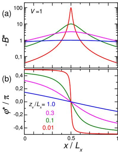
FIG. 2. (Color online). (a) Abrikosov vortex-induced stray fields,  $-B^*(x)$ , at four different distances  $z_v$  of the vortex to the junction and at  $x_v = 0.5L_x$  (in the semi-logarithmic scale). The minus sign is due to the opposite sign of the vortex stray field with respect to the vortex. (b) Corresponding Josephson phase shifts  $\varphi^*(x)$ .
