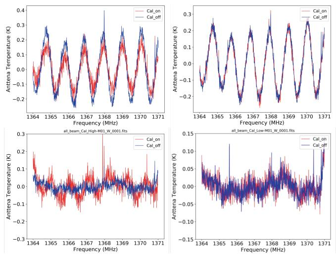
FIG. 15.— The comparison of the band-pass ripples before (upper panel plots) and after (lower panel plots) the cabin dock platform is covered with metal mesh. The left side plots are with high power noise diode injection and the right side plots are with the low noise power.
