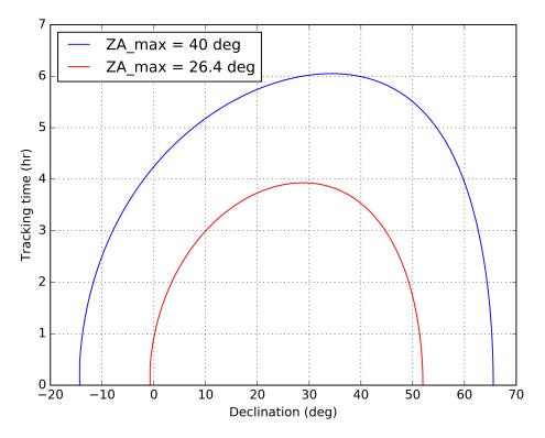
FIG. 20.— Maximum tracking time for source at specific declination. Results for zenith angle of  $40^{\circ}$  and  $26.4^{\circ}$  are represented with blue and red color, respectively.
