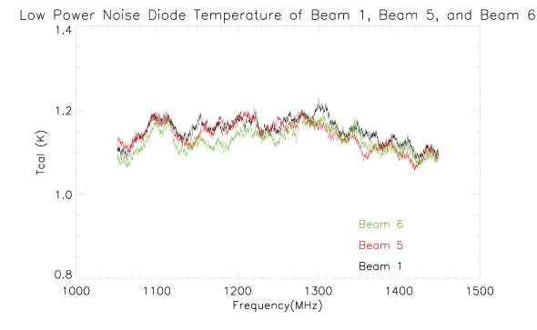
FIG. 1.— The low power noise diode temperatures of Beam 1, Beam 5, and Beam 6. The 3 beams plotted here are representative of the rest. The data for all 19 beams and polarizations is available and is being used for subsequent calibration.
