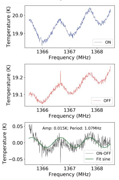
FIG. 17.— Standing wave test from the ON/OFF observation towards J073631.82+383058.3. The top and middle panels are the calibrated band-passes from ON- and OFF- position. The bottom panel is the ON-OFF calibrated band-pass with a linear baseline removal. The sine function is fit to the spectrum, which gives the amplitude of the standing wave  $\sim 15$  mK.
