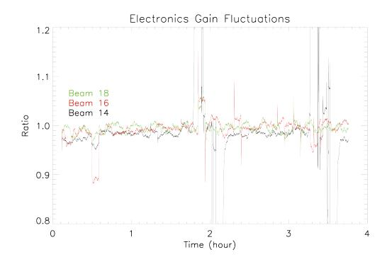
FIG. 3.— The electronics gain fluctuations of the system over several hours. The vertical shows the ratio of fluctuations with respect to the mean temperature over time of Beams 14, 16, and 18. The three beams presented here represent the strongest electronics gain fluctuations out of all 19.
