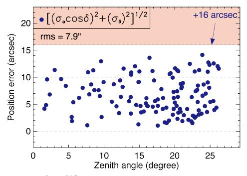
FIG. 10.— Pointing error  $[(\sigma_{\alpha} \cos \delta)^2 + (\sigma_{\delta})^2]^{1/2}$  verseus zenith angle for the 19-beam receiver of FAST. 2017).
