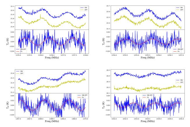
FIG. 18.— Bandpass spectrum at different frequency ranges during ON-OFF observations towards NGC 2718. The amplitudes of standing wave in frequency range of [1150,1158],[1254,1257], [1367,1370] and [1432,1435] MHz are 15, 11, 22, and 9.5 mK, respectively.
