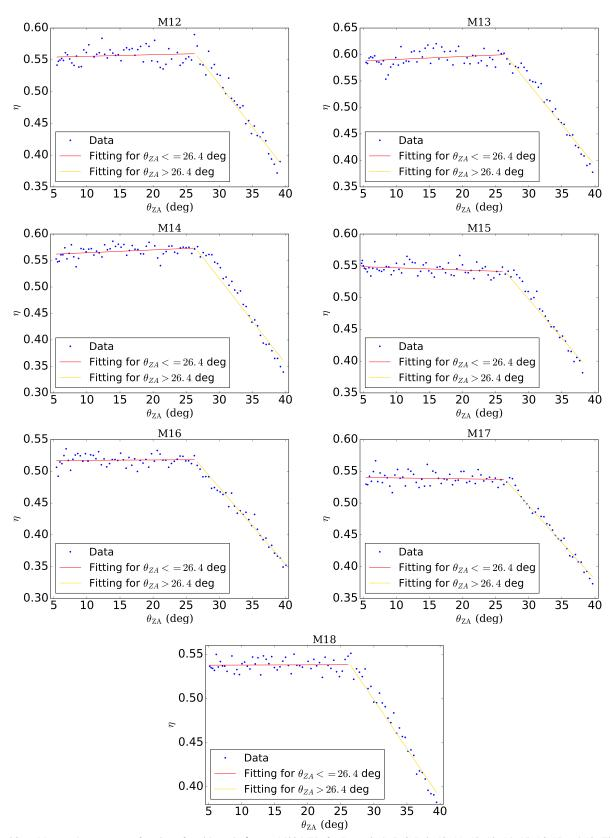
FIG. 28.— Measured  $\eta$  curve as a function of zenith angle  $\theta_{ZA}$  at 1400 MHz for Beam 3, 4, 5, 6, 7, 9, 10, 11, 12, 13, 14, 15, 16, 17 and 18. Fitting results when  $\theta_{ZA} \leq 26.4^{\circ}$  and  $\theta_{ZA} > 26.4^{\circ}$  are represented with red and gold solid line, respectively.
