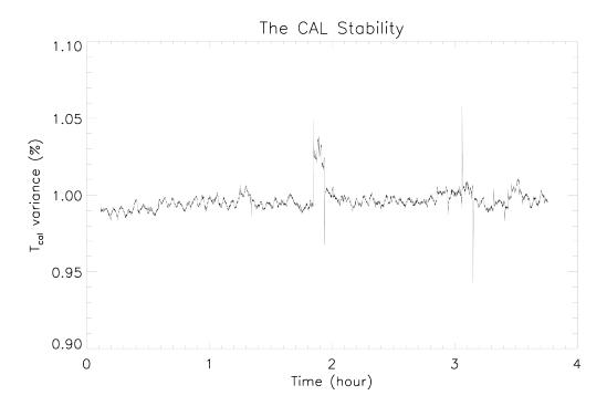
FIG. 4.— The noise diode stability. An upper limit on the noise diode stability as a function of time measured by monitoring the median value of the electronics gain in all 19 beams during hot load measurements.
