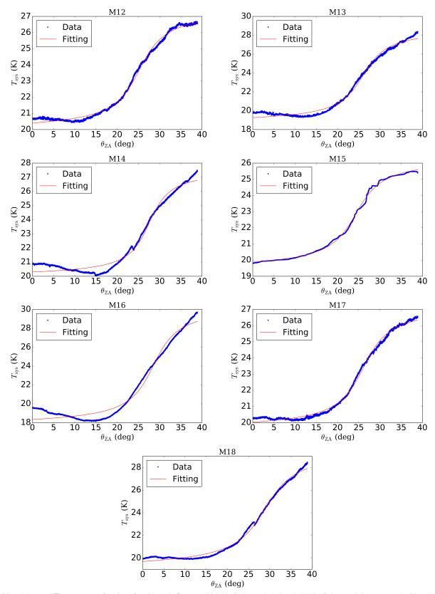
FIG. 29.— Measured  $T_{\rm sys}$  curve as a function of zenith angle  $\theta_{\rm ZA}$  at 1400 MHz for Beam 1, 2, 8 and 19. The fitting result is represented with red solid line.
