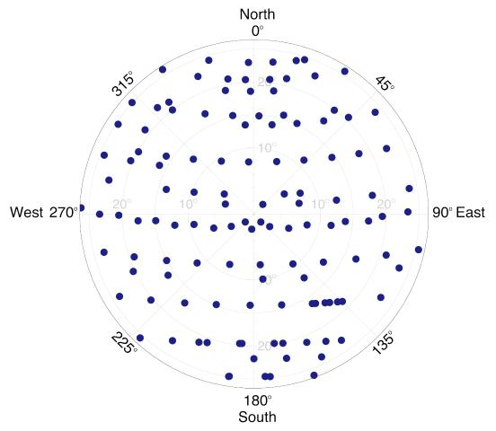
FIG. 9.— Distributions of the observed pointing calibrators in the sky coverage of FAST with full gain (zenith angle  $\leq 26.4^{\circ}$ ). The observation period is from February 16 to March 15, 2019. In this plot, the zenith angle is from 0° to 26.4° as indicated by grey circles, the azimuth angle is from 0° to 360°. The directions marked in the periphery of the plot are the geographic north, east, south and west at the FAST site.
