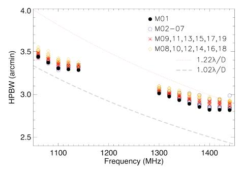
FIG. 8.— Half-power beamwidth (HPBW) verseus observation frequency for the 19-beam receiver of FAST. The target source is 3C454.3. The observation date is December 17, 2018. The beamwidths corresponding to the frequency range of 1160-1280 MHz can not be well fitted, as the strong RFI appear during the observation.
