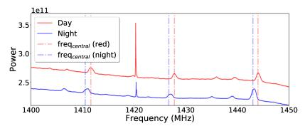
FIG. 26.— Zooming in the X and Y axes in the Fig. 25, the systemic shift of this wide RFI is plotted. Red lines represent daytime and blue lines represent nighttime. The vertical dash dot line shows the center frequency of a single RFI signal, making it easy to see the amplitude of the frequency shift from day to night.
