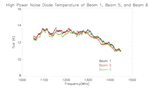
FIG. 2.— The high power noise diode temperatures of Beam 1, Beam 5, and Beam 6. The 3 beams plotted here are representative of the rest. The data for all 19 beams and polarizations is available and is being used for subsequent calibration.
