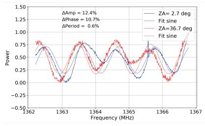
FIG. 16.— Band-pass ripples at different zenith angles. The blue line is the spectrum obtained with drift-scan observation at  $ZA = 2.7^{\circ}$  and the red line is at ZA = 36.7°. The dashed lines are the sine function fitting results. A linear baseline removal was processed before hand. The intensity of the spectra are normalized and the unit is relative power.
