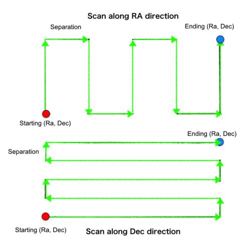
FIG. 21.— Schematic diagram of OTF mode. The blue line represents scanning trajectory. The top and bottom figure shows scan information along RA and Dec direction, respectively.
