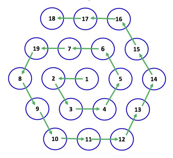
FIG. 22.— Schematic diagram of MutiBeamCalibration mode. Green arrow line represents the beam sequence for observing the calibrator. In this plot, the 5. SUMMARY
