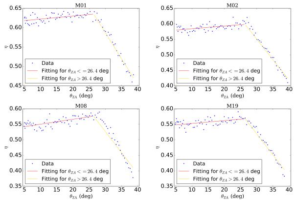
FIG. 11.— Measured  $\eta$  curve as a function of zenith angle  $\theta_{ZA}$  at 1400 MHz for Beam 1, 2, 8 and 19. Fitting results when  $\theta_{ZA} \le 26.4^{\circ}$  and  $\theta_{ZA} > 26.4^{\circ}$  are represented with red and gold solid line, respectively.
