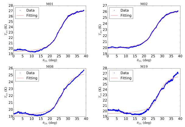
FIG. 12.— Measured  $T_{\rm sys}$  curve as a function of zenith angle  $\theta_{\rm ZA}$  at 1400 MHz for Beam 1, 2, 8 and 19. The fitting result is represented with red solid line.
