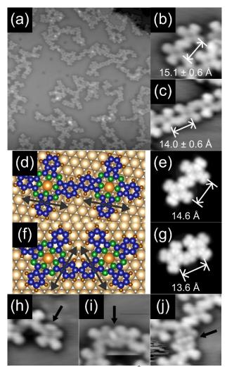
FIG. 1. (a) Annealed 0.25-ML CuPc on Cu(111) (500×500 Å<sup>2</sup>). Specific parallel (b) and angular (c) bonding orientations ( $50\times50$  Å<sup>2</sup>). Atomic model (d) and STM simulation (e) of parallel bonding. Atomic model (f) and STM simulation (g) of angular bonding. (h)-(j) Different CuPc-Cu adatom coordination structures ( $50\times50$  Å<sup>2</sup>). STM simulations at +0.9 V. Imaged +0.9 V and 0.5 nA.
