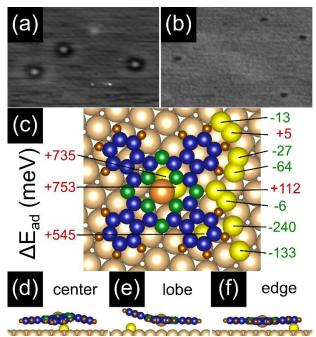
FIG. 6. Surface defects on Cu(111) before (a) and after (b) a tip change (-1,2 V, 0.2 nA,  $120 \times 80 \text{ Å}^2$ ) (c) Relative adsorption energies of CuPc near and on top of S defects. (d)-(f) Three relaxed geometries of CuPc by S on Cu(111).
