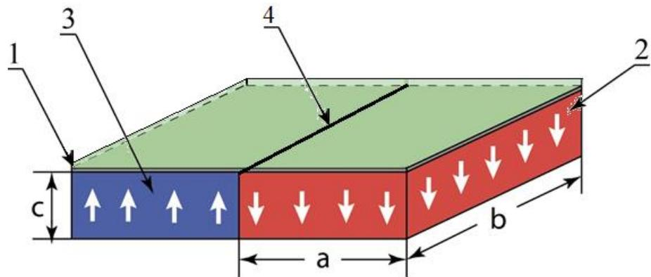
Fig. 3. The schematic image of the system of two NdFeB permanent magnets. 1 – cover glass; 2 – NdFeB permanent magnet with up orientation of magnetization as indicated by white arrows; 3 – NdFeB permanent magnet with down orientation of magnetization as indicated by white arrows; 4 – contact surface of two NdFeB permanent magnets;  $a=23$  mm,  $b=30$  mm,  $c=10$  mm.
