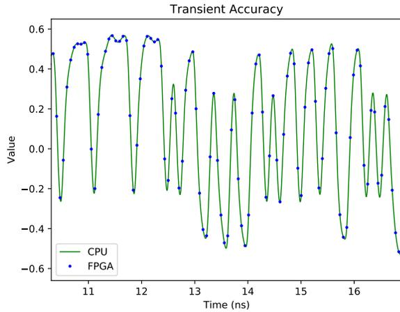
**Figure 9: Comparison of FPGA emulation and CPU simulation waveforms, shown at the output of the RX CTLE. Our emulator evaluates analog signals only on digital clock edges, and these samples are shown as dots. The continuous-time waveform was calculated using CPU simulation and is shown as a solid curve. Over all 160 combinations of TX and RX equalizer settings, the worst-case relative error observed was  $-0.7\%/+1.1\%$ .**
