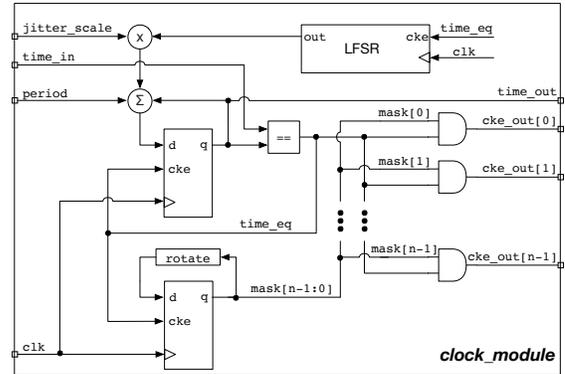
Figure 7: Clock module used to model TX and RX clock behavior. During each emulation cycle,  $time\_in$  is compared to  $time\_out$ . If they match,  $time\_out$  is incremented and one of the  $cke\_out$  signals is asserted. The clock phase is advanced by rotating mask, and jitter is implemented by adding the scaled output of an LFSR to the period input.
