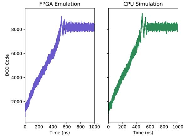
**Figure 10: Startup transient of the high-speed link transceiver captured by the FPGA emulator. The RX DCO code is shown over the first 1  $\mu\text{s}$  of operation, starting from an initial value of 1000 (7.6 GHz) and settling around 8192 (8.0 GHz).**
