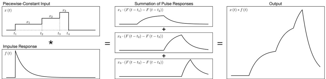
**Figure 2: The response of a linear time-invariant (LTI) system to a piecewise-constant input can be computed as a summation of pulse responses, each dependent on two values of the system's step response  $F(t)$ .**
