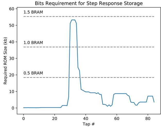
**Figure 8: Number of bits required to store step response data for each tap in the analog dynamics engine (ADE). Memory on the Xilinx Zynq-7045 FPGA used in our implementation can be allocated in increments of a half BRAM tile (18 kb) as indicated by the dashed lines. Only 8% of taps required more than the minimum increment.**
