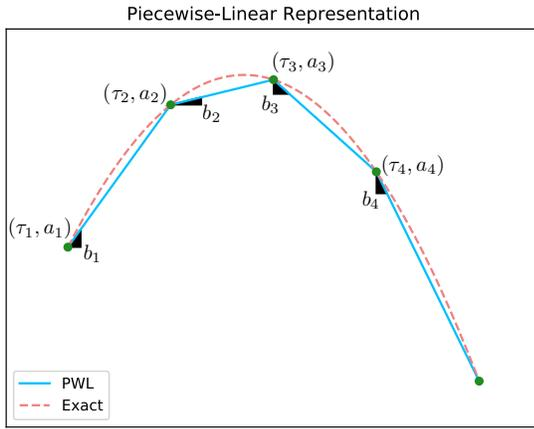
Figure 6: Our emulator uses piecewise-linear lookup tables to store step responses and nonlinear functions in a compressed form. Each time point  $\tau_k$  in the lookup table is assigned an offset  $a_k$  and a slope  $b_k$ .
