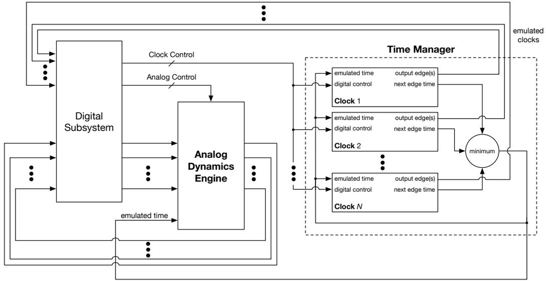
**Figure 1: The proposed emulator architecture. A digital subsystem generates piecewise-constant analog inputs for an analog dynamics engine (ADE) whose outputs are computed as superpositions of pulse responses. A time manager moves emulated time forward from one emulated clock edge to the next and generates clocks for the digital subsystem.**
