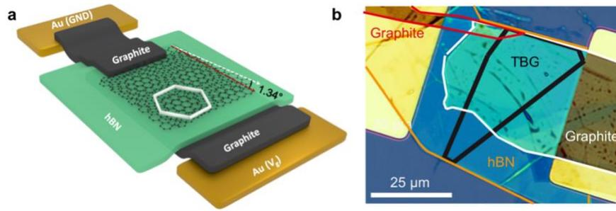
**Figure 1 | Device layout.** **a** Sketch of the van der Waals stack with TBG on top of hBN and a bottom graphite electrode. The TBG is contacted by a graphite stripe. **b** Optical micrograph of the device with boundaries of the different layers indicated as guide to the eye. Details of the device fabrication are given in methods and Supplementary Information.
