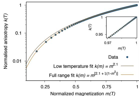
FIG. 4. (Color Online) Simulated temperature dependence of the anisotropy for L1<sub>0</sub>-FePt in a nearest-neighbor approximation. Lines show fits for the low-temperature exponent  $l = 2.1$  and an expanded fitting  $l = [2.1 + \xi(1 - m^2)]$ , where  $\xi = 0.162145 \pm 0.000437$ , valid over the whole temperature range. Inset displays the scaling in the low-temperature region.
