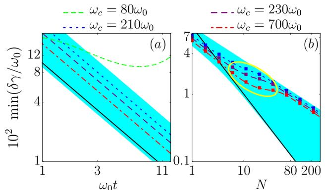
FIG. 2.  $\min(\delta\gamma)$  as a function of (a) time and (b) average photon number with different  $\omega_c$ s. The black lines denote the weak HL. The shaded areas in panels (a) and (b) are bound by the SNL (upper bound) and the ideal-case-promised precision (lower bound) in the absence of noise.  $N = 10$  in panel (a),  $t = 10\omega_0^{-1}$  in panel (b), and the other parameters used are the same as those in Fig. 1.
