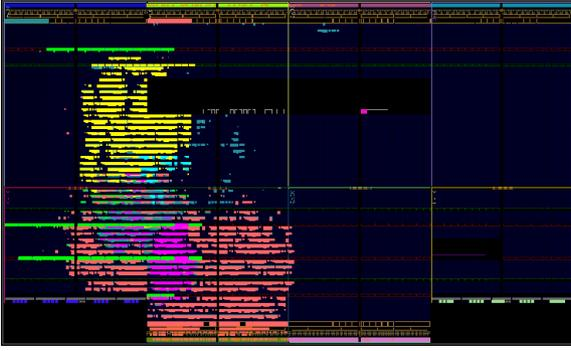
**Fig. 9** The implementation result of RVSoC on a xc7a100tcs324-1 FPGA.
