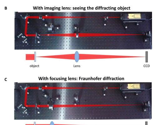
**Figure 2:** Different operation modes of the setup, for (A) direct Fresnel diffraction, (B) imaging the sample on the camera and (C) Fraunhofer diffraction. The modes A and B are the most useful for the demonstrations, the Fraunhofer diffraction (C) can be often skipped.
