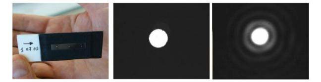
**Figure 4**. Pictures of the diffraction by a hole experiment. (Left) holes sample. (Center) Image of a single hole and (Right) its Fresnel diffraction pattern showing the Airy rings surrounding the center spot.
