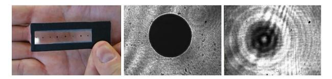
**Figure 3**. Pictures of the Fresnel-Arago diffraction experiment. (Left) black disks sample. (Center) Image of a black disk and (Right) its Fresnel diffraction pattern showing a bright spot in the shadow center.
