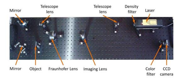
Figure 1: Experimental demonstration setup, see text for details
