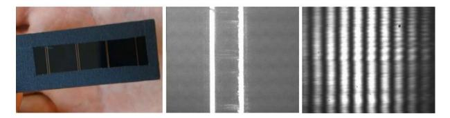
**Figure 5**. Pictures of Young's interferences experiment. (Left) Double slits sample. (Center) Image of a double slit and (Right) its interference pattern.
