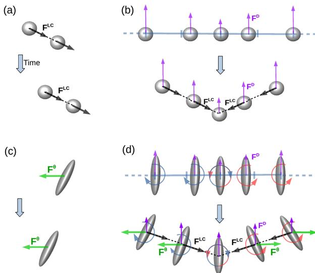
FIG. 1. **Schematic of competing mechanisms:** (a)  $F^{LC}$  acts on the pair along line joining their centers leading to horizontal drift. (b) Clumping of array of spheres result from the line of centres force  $F^{LC}$ , acting along with reduced drag force  $F^D$ . (c) A spheroid drifts laterally as it falls when it is oriented obliquely with respect to gravity (d) Lateral drift  $F^\theta$  competing with the clumping induced by  $F^{LC}$  and  $F^D$ .
