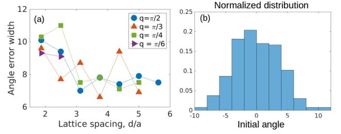
FIG. 8. **Error in initial orientation:** (a) The error is quantified by  $0.5 \times (\text{maximum} - \text{minimum})$  of the initial angles in any given run. This measure of the width in release angle is plotted here as a function of lattice spacing for  $qd = \pi/2, \pi/3, \pi/4$  and  $\pi/6$ . (b) a combined distribution of, initial angles of several experimental runs for a fixed  $qd = \pi/2$  and  $d = 3.75a$ .
