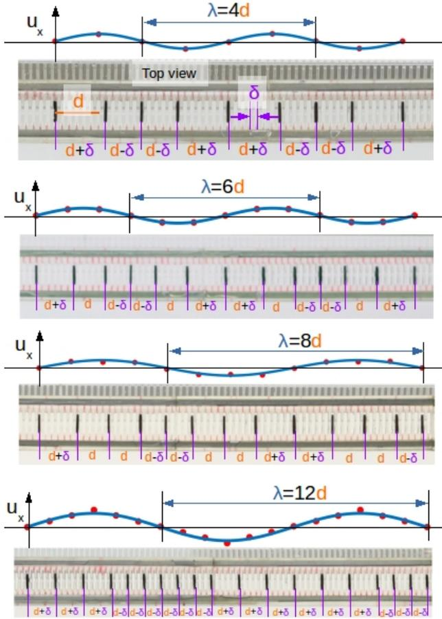
FIG. 7. **Release mechanism:** Top view of the release mechanism shown before release, with the disks loaded in the slots. The centre-to-centre distance between adjacent slots is  $\delta$  and the lattice spacing of reference lattice is  $d$ . Initial horizontal positional perturbation  $u_x$  are shown by fitting a sine function (blue curve) to the measured perturbations (red dots) for the wavelengths  $\lambda = 4d, 6d, 8d$  and  $12d$ .
