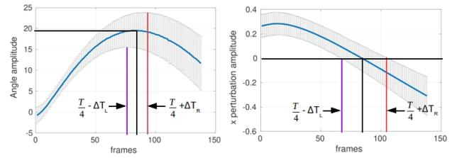
FIG. 9. **Frequency measurement:** Amplitude of the fitted sine wave plotted for the angle and the horizontal positional perturbations, along with the residual error of the fit shown as vertical error-bar at each frame. At quarter time period of the wave, the amplitude of angle peaks and the horizontal perturbation crosses  $y = 0$  axis, consistent with our theory.
