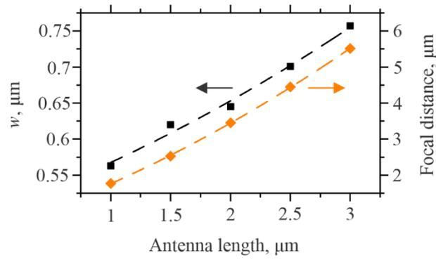
**Figure 5.** Dependences of the beam width at the focal position (squares) and of the focal distance (diamonds) on the length of the antenna calculated for spin waves with the wavelength of  $0.6 \mu\text{m}$ . Dashed curves are guides for the eye.
