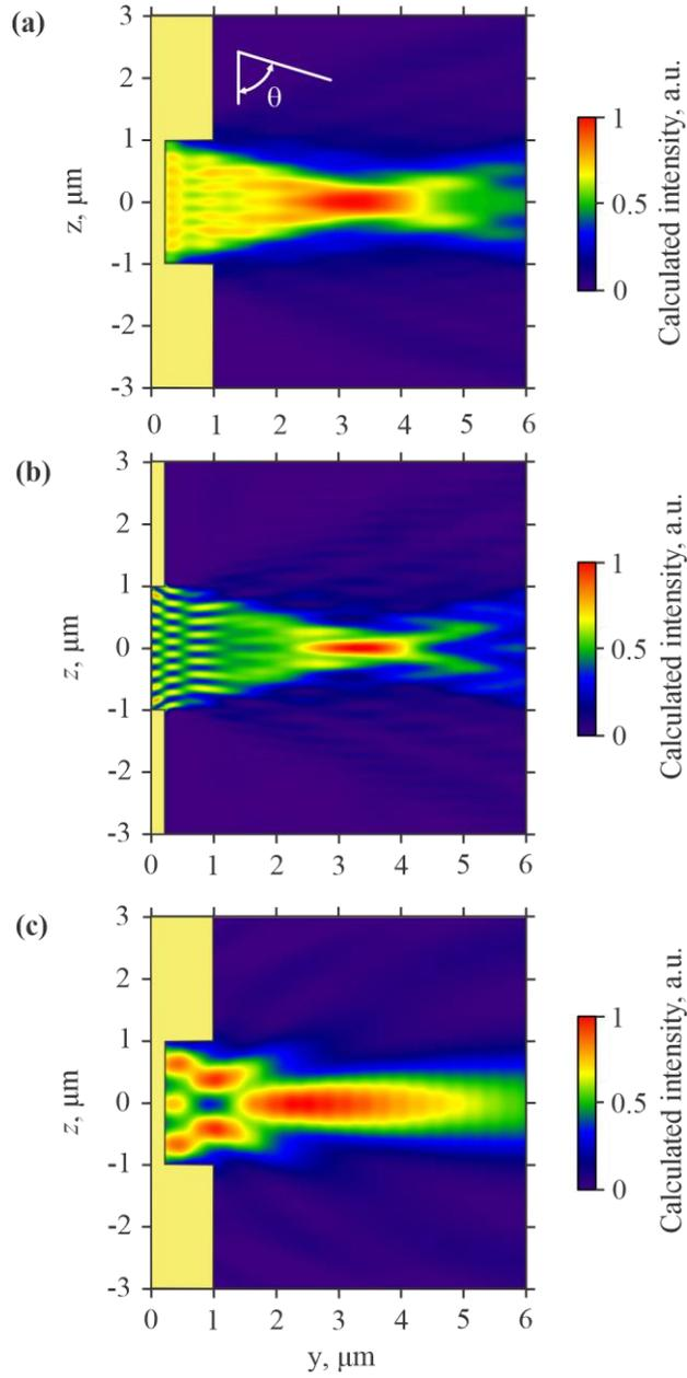
**Figure 3.** (a) Calculated intensity map of spin waves radiated by the antenna. The schematic of the antenna and the connecting microwave lines is superimposed on the map. (b) Calculated intensity map of spin-wave diffraction from a one-dimensional slit. Superimposed rectangles mark the regions with an increased damping. (c) Similar to (a) calculated for the case of isotropic spin-wave dispersion. Calculations were performed for  $H=500$  Oe and  $f=3.8$  GHz.
