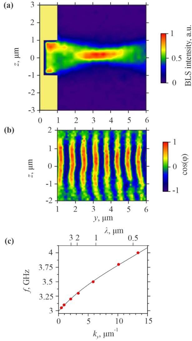
**Figure 2.** Representative spatial maps of the intensity (a) and phase (b) of radiated spin waves recorded by BLS at  $H=500$  Oe and  $f=3.8$  GHz. (c) Measured (symbols) and calculated (solid curve) dispersion curve of spin waves.
