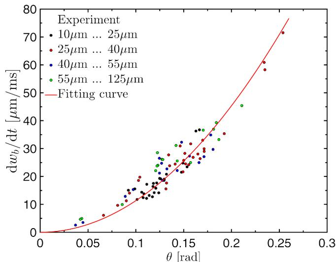
**Fig. 7** Growth rate of the bridge width in dependence of the contact angle. The different colors in the experimental data visualize different diameter ranges of the merged (final) droplets. Since the profile of the bridge does not vary much during the coalescence, one can fit a quadratic curve to the width characteristics as well (solid red curve), the ratio of bridge height and width is roughly constant, between 0.045 and 0.06 (see Fig. 9)
