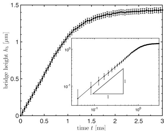
**Fig. 4** Measured bridge height  $h_b$  during the merging process of two nearly equal-sized droplets ( $D_{01} = 35.5 \mu\text{m}$ ,  $D_{02} = 34.7 \mu\text{m}$ ,  $H_{01} = 1.13 \mu\text{m}$ ,  $H_{02} = 1.10 \mu\text{m}$ ,  $\theta = 7.3^\circ$ ).
