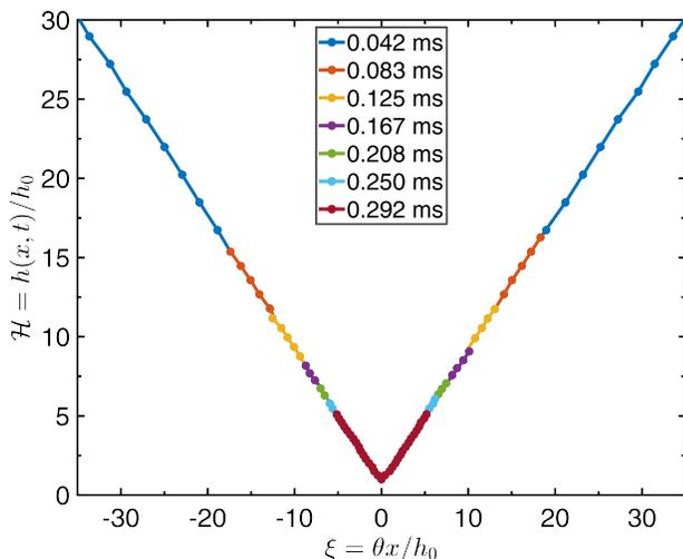
**Fig. 8** Scaled height profile at different instants at the position of the bridge center ( $x=0$ ), all curves collapse to one single curve, which verifies the self-similarity of the height profile ( $D_{0_1} = 65.5 \mu\text{m}$ ,  $D_{0_2} = 101.8 \mu\text{m}$ ,  $H_{0_1} = 1.41 \mu\text{m}$ ,  $H_{0_2} = 2.19 \mu\text{m}$ ), from the center of the bridge we plotted the profile 12 micrometer in both directions
