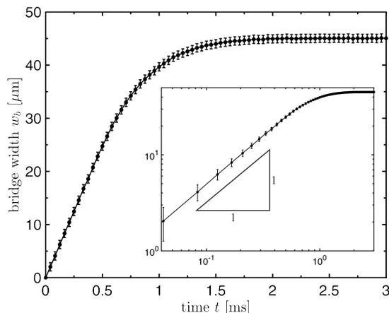
**Fig. 5** Measured bridge width  $w_b$  during the merging process of two nearly equal-sized droplets ( $D_{01} = 35.5 \mu\text{m}$ ,  $D_{02} = 34.7 \mu\text{m}$ ,  $H_{01} = 1.13 \mu\text{m}$ ,  $H_{02} = 1.10 \mu\text{m}$ ,  $\theta = 7.3^\circ$ ).
