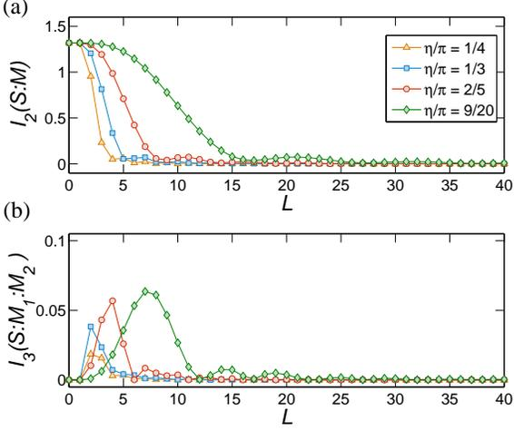
FIG. 2: The  $L$  dependence of BMI (a) and TMI (b) for various transmission angle  $\eta$  of the BS. The input state of each mode is vacuum state. The transmission angles of the BS are  $\eta = \pi/4$  (triangles),  $\pi/3$  (squares),  $2\pi/5$  (circles) and  $9\pi/20$  (diamond), respectively.
