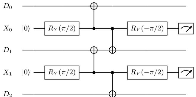
Figure 2. Circuit diagram for one error correction cycle of the distance-3 phase flip code. The  $XX$ -parity checks are implemented by coupling to ancillas, which are subsequently measured to give the syndrome information.
