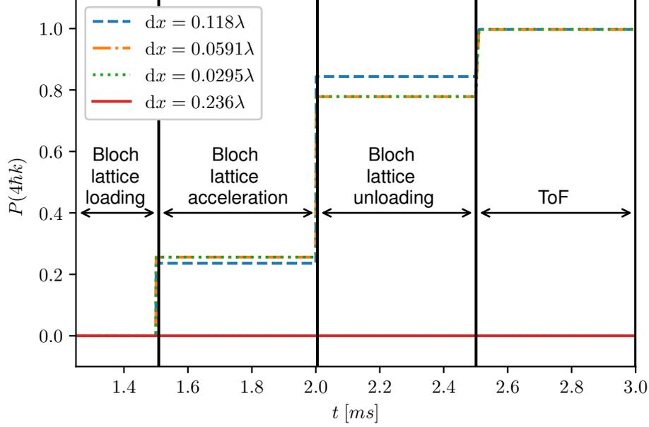
**Figure 9.** Numerical convergence of a simulated  $(2+2)\hbar k$  Bragg+Bloch beam splitter in a waveguide. We analyse the numerical convergence behaviour when changing the position step  $dx$  of the numerical simulation using the third-order split-operator method. The same parameters as Fig. 8 are used. At a time step of  $dt = 10^{-6}$  s, the simulation converges well for a position step of  $dx \approx 0.06\lambda$ .
