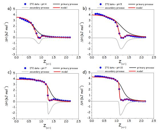
*Figure 6*. Binding isotherms for PDADMAC in sodium alginate titrations at pH (a) 4, (b) 5, (c) 7, and (d) 10 for Type I experiments at 25 °C. The uncertainty in the determination of the fitting parameters is approximately 5%.
