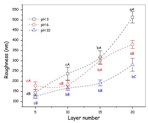
**Figure 8.** Roughness of films according to interferometric confocal microscopy of the PDADMAC and sodium alginate films produced at pH 3, 6, and 10 with 5, 10, and 20 layers. Equal lower case letters show that for the same pH, the results did not differ according to the Tukey test at a 5% significance level. Equal capital letters show that on the same layer, the results did not differ according to the Tukey test at a 5% significance level.
