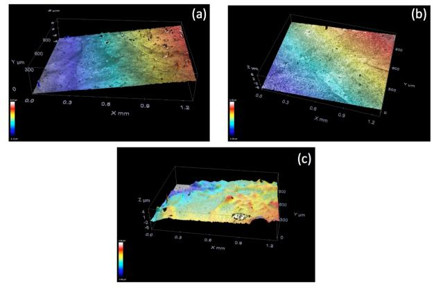
**Figure 9.** 3D representative topographical image of films from the 20<sup>th</sup> layer by interferometric confocal microscopy of PDADMAC and sodium alginate films deposited at (a) pH 10, (b) pH 6, and (c) pH 3.
