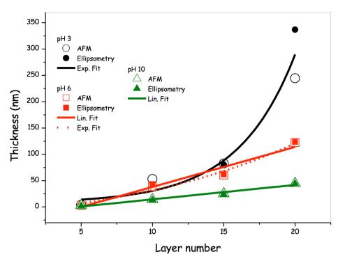
**Figure 7.** Growth regime of PDADMAC and sodium alginate films at pH 3 ( $R^{2}_{AFM} = 0.92$  and  $R^{2}_{El.} = 0.98$ ), pH 6 ( $R^{2}_{AFM, lin.} = 0.97$  and  $R^{2}_{El., lin.} = 0.94$ ;  $R^{2}_{AFM, exp.} = 0.98$  and  $R^{2}_{El., exp.} = 0.92$ ), and pH 10 ( $R^{2}_{AFM} = 0.98$  and  $R^{2}_{El.} = 0.96$ ).  $R^{2}$ , El., lin., and exp. denote the coefficient of determination, ellipsometry, linear, and exponential, respectively.
