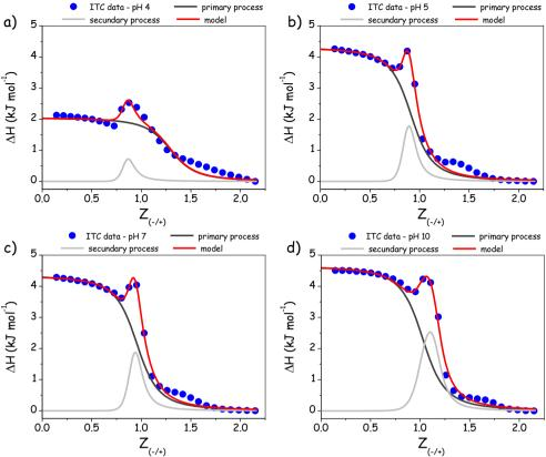
*Figure 5.* Binding isotherms for sodium alginate in PDADMAC titrations at pH (a) 4, (b) 5, (c) 7, and (d) 10 for Type II experiments at 25 °C. The uncertainty in the determination of the fitting parameters is approximately 5%.
