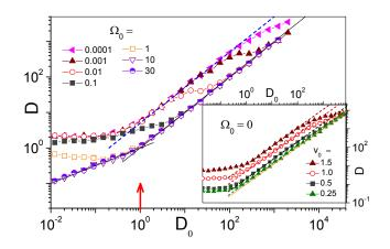
FIG. 6: Diffusion, D, vs. translational noise,  $D_0$ , in the cellular flow of Eq. (1) for  $D_{\theta} = 0$  and main panel:  $v_0 = 1$  and different  $\Omega_0$ , inset:  $\Omega_0 = 0$  and different  $v_0$  (see legends). Other model parameters are:  $\alpha = 1$ ,  $U_0 = 1$ ,  $L = 2\pi$ . Straight lines represent the analytical predictions discussed in the text for high (solid) and low chirality (dashed). A vertical arrow locates  $D_0 = D_L$ .
