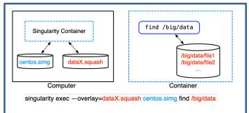
Figure 1. Data and information flow when using SquashFS + Singularity to access bundled datasets. A container (dashed lines) is started with the singularity command, and its image is provided by the normal file "centos.simg". The SquashFS filesystem file "dataX.squash" is mounted in the container at launch time. Within the container, the Linux command run is "find /big/data", which access the data files normally under the mountpoint "/big/data".
