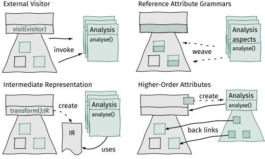
**Figure 1** Different approaches for implementing static analysis.
