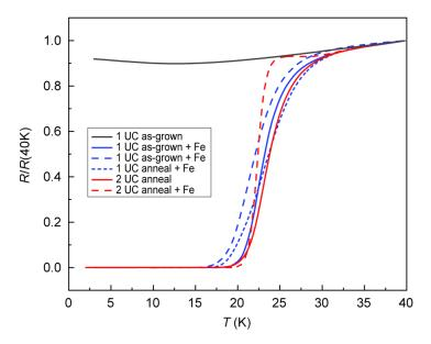
FIG. 5. Summary of transport measurement results of different samples in this work. The anneal was carried out at 480 °C for 3 hours. All samples were capped by 12-UC FeTe.
