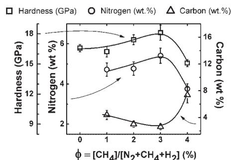
Figure 3. Hardness and nitrogen concentration (left axis) and carbon concentration (right axis) at 200 nm surface samples with different  $\text{CH}_4$  content in the gaseous mixture feeding the chamber.
