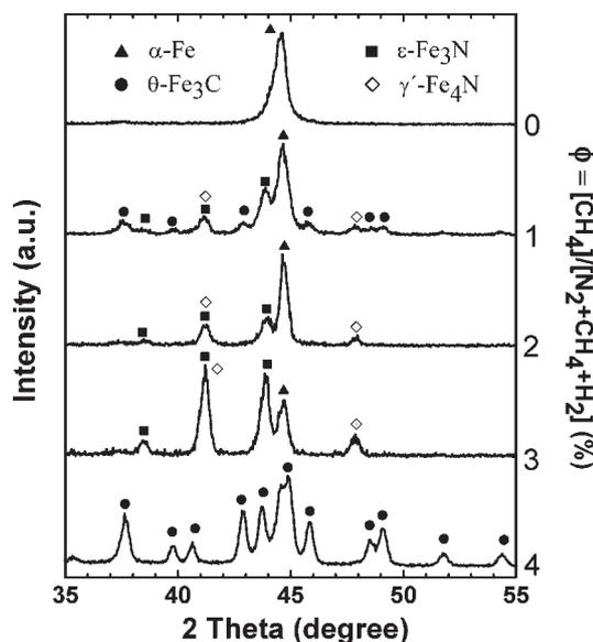
Figure 1. XRD pattern of the nitrocarburized samples as a function of the  $\text{CH}_4$  content in the plasma atmosphere.
