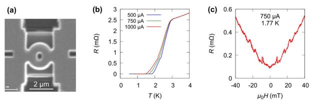
Supplementary Figure 4. Results of Ring D. (a) Scanning ion microscope image. (b) Resistance as a function of temperature R(T). (c) Resistance as a function of magnetic field R(H) at a temperature in the transition region. The amplitude of the magnetoresistance oscillations is much smaller than those of the rings without the extrinsic phase e.g. Ring A (see Fig. 5 in the main text).
