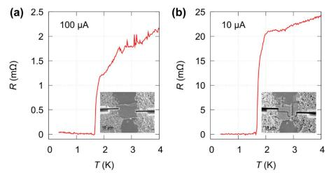
Supplementary Figure 1. Resistance as a function of temperature R(T). (a) R(T) before and (b) after ring structuring (Ring A). The zero-resistance  $T_c$  is unchanged by the ring structuring.
