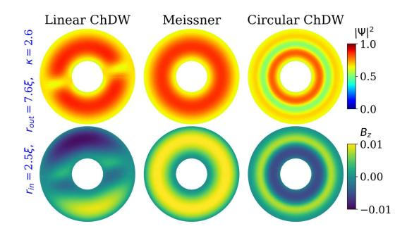
Supplementary Figure 3. Contour plots of the total Cooper-pair density and the magnetic induction for different states of Supplementary Figure 2a.
