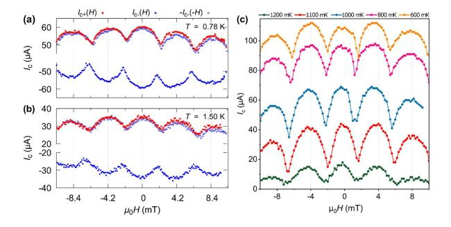
**Figure 4 | SQUID oscillations observed in the Sr**<sub>2</sub>**RuO**<sub>4</sub> **microrings.** (a) Critical current as a function of magnetic field  $I_c(H)$  of Ring A measured at 0.78 K and 1.50 K. The open blue circles show time-reversed critical current. (c)  $I_c$  oscillations in Ring B over a wide range of temperatures. The  $I_c$  values were obtained from I(V) measurements at each magnetic field. The rings were heated up to above 5 K between each magnetic field.
