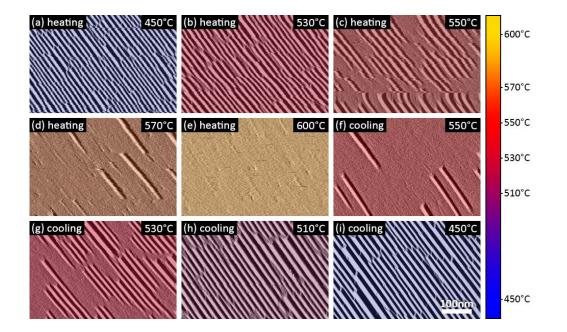
Figure 4. Fully reversible Ge nanoripple formation on  $8^{\circ}$  vicinal Si (100) with miscut towards (110), as seen by *in vivo* high-temperature STM images recorded during temperature ramping from 450° to 600°C (a-e) and cooling back to 450°C (g-i). The Ge coverage was 4.7 ML.
