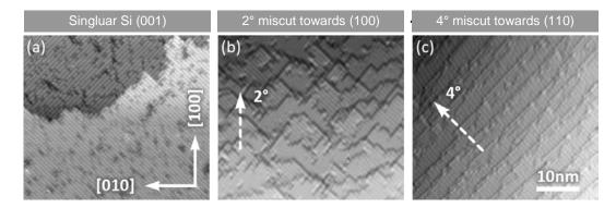
**Figure 1. Step structure** of the initial singular and miscut vicinal Si (001) surfaces as imaged by STM. The miscut angle varies between  $0^\circ$ ,  $2^\circ$  and  $4^\circ$  from (a) to (c), respectively, and its direction changes from towards (100) in (b) to towards (110) in (c) as indicated by the dashed arrows. The scale is the same for all images.
