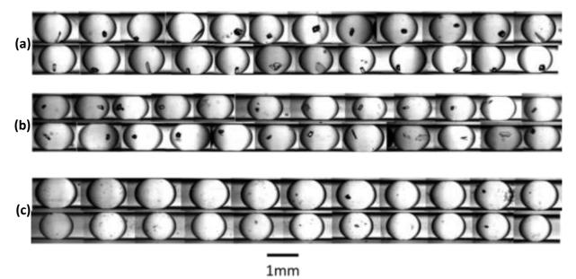
Figure 3: Micrographs of droplets at the end of the experiment of crystallization of Sulfathiazole in water (a) droplets generated at 70°C ( $C_i$ =5.87mg/mL), (b) droplets generated at 55°C ( $C_i$ =2.64mg/mL), (c) droplets generated at 45°C ( $C_i$ =1.56mg/mL).
