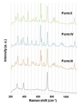
Figure 6: Different Raman spectra observed for crystals of Sulfathiazole polymorphs in water in 1mm droplets. The bottom curve corresponds to a reference spectrum of a supersaturated droplet without crystals.
