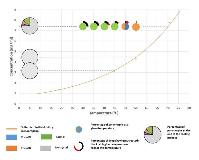
*Figure S3: Graphical summary of polymorphs obtained during cooling crystallization, to* 10°C by steps of 5°C every 5 hours, *of Sulfathiazole in isopropanol.*
