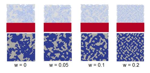
**Figure 5**: Upper panels: side view of the RVEs for all composite microstructures considered in this work. Lower panels: morphology of the composites at the gripper-object interface.
