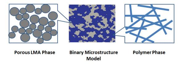
**Figure 1**: Schematic illustration of the porous-LMPA-PDMS composite. The porous LMPA phase is composed of sintered LMPA powders with tunable porosity, which enables tunable physical properties of the phase including thermal expansion, stiffness and density. Both the LMPA phase and the PDMS matrix phase are percolating in 3D, forming an interpenetrating bi-continuous microstructure (middle panel).
