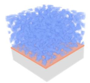
**Figure 4**: 3D visualization of a representative volume element (RVE) for the gripper-composite interface, which includes a cubic composite microstructure associated with w = 0.2 and linear dimension of 100  $\mu$ m, a homogeneous gripped sample (light gray) and the virtual interface (light red). We note that the interface in our simulations is treated as a layer of bonds with distinct mechanical properties from those associated with different materials.
