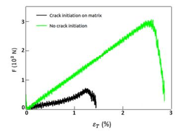
**Figure 7**: Reaction force as a function of tensile strain  $\varepsilon_{\rm T}$  for the prefect interface case (green curve) and the cracked interface case associated with a 0.5% thermal strain (black curve). The gripper is composed of a LMPA/PDMS composite with w = 0.2 (see Fig. 8).
