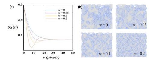
**Figure 3**: (a) Parametrized damped oscillation two-point correlation functions  $S_2$  for modeling LMPA-PDMS composites. (b) 3D virtual composite microstructures associated with different correlation functions obtained with stochastic reconstruction. The LMPA phase is shown as light gray (with interface shown in light blue for better visualization effect) and the PDMS matrix is transparent. The linear size of the reconstructed composite microstructure is 100  $\mu$ m.
