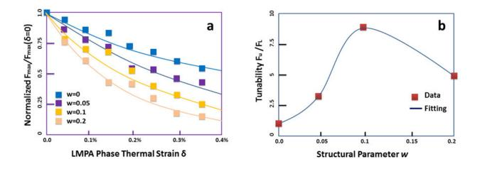
**Figure 9**: (a)  $F_{\text{max}}^L/F_{\text{max}}^U$  as a function of  $\delta$  up to 0.5% volumetric thermal strain for different composite microstructures. (b) The contrast of  $F_{\text{max}}^U$  and  $F_{\text{max}}^L$  at  $\delta = 0.5\%$  for different composite microstructures.
