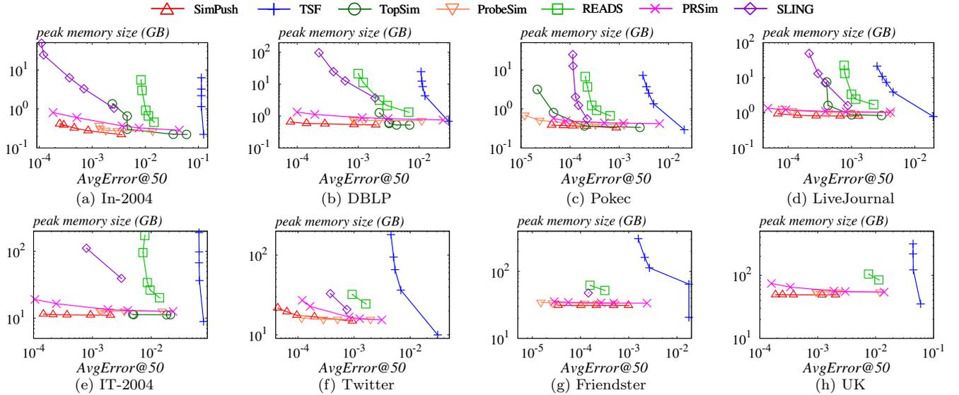
Figure 6: Average error *vs.* peak memory usage.
