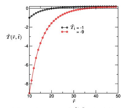
Figure 4.6: Angularly averaged temperature profile  $\tilde{T}(\tilde{r}, \tilde{t})$  vs. the radial distance  $\tilde{r}$  from the colloid center. Results correspond to a small ( $\tilde{T}_1 = -1$ ) and a deep ( $\tilde{T}_1 = -9$ ) quench. For the deep quench, the temperature field attains negative value ( $\tilde{T}(\tilde{r}) < T_c$ ) over a much larger distance from the colloid. This has an impact on the local structure formation process.
