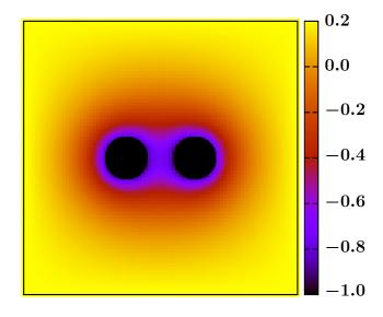
Figure 4.7: Temperature profile of the two colloid system at an early time  $\tilde{t} = 2$  in the midplane (z = L/2) of the system. Both colloids are quenched to a temperature  $\tilde{T}_1 = -1$  and the initial temperature is  $\tilde{T}_0 = 0.2$ . The temperature at the outer boundaries of the box is kept fixed at  $\tilde{T}_0 = 0.2$ . A large temperature gradient is established and the temperature fields of the two colloids get coupled with each other.
